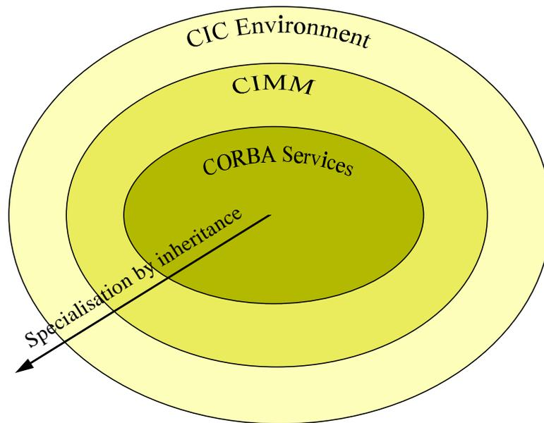
FIG. 4: The CIMM as a bridge between CORBA and CIC environments.
