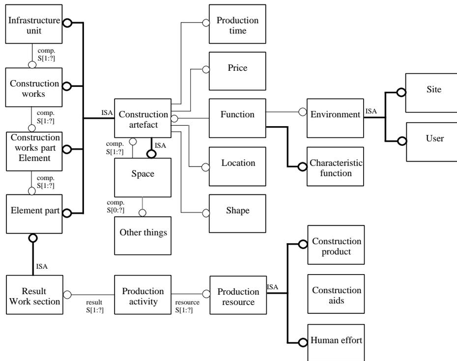
FIG. 20: Level order and main properties of construction works
