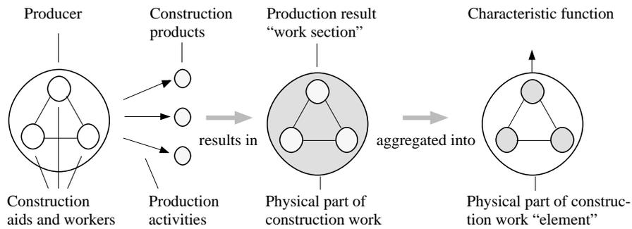
FIG. 14: A work section is the result of production activities on construction products
