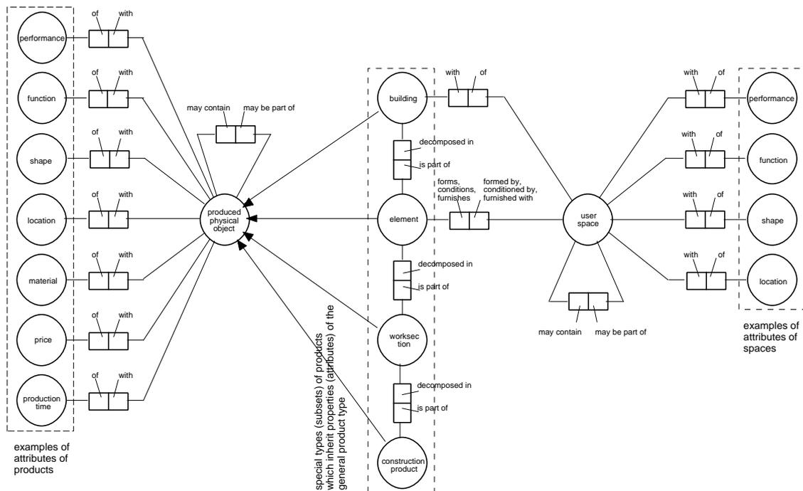
FIG. 19: Schema in the ISO Technical Report relating basic construction information concepts
