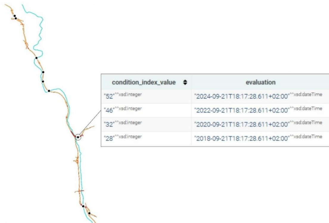
Figure 23: Bridge condition index evolution over time.
