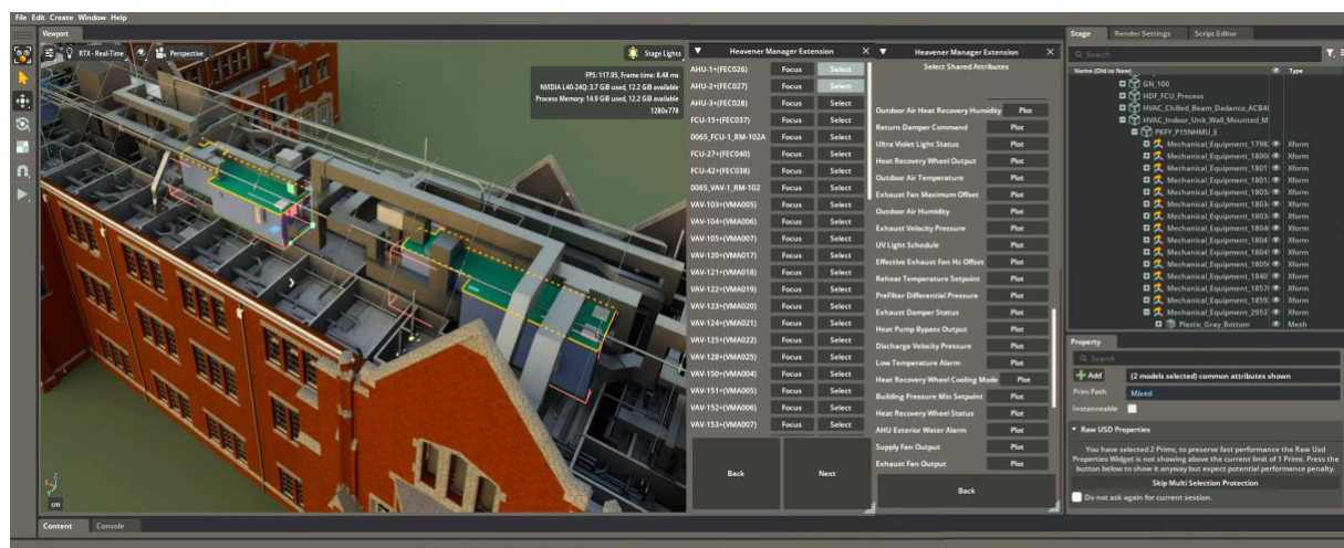
Figure 6: Device inspection and trends interface in Omniverse DT.
