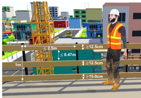
Figure 1: Guardrail protection rule in Denmark (HÅNDBOGEN, 2025).
