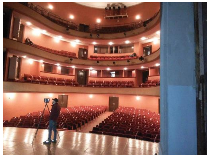
Figure 5: Reality capture, FARO FocusS350 adjustment during the recording of interior spaces of the main auditorium in Mahieddine Bachtarzi Theatre. (Source: Author, 2022).
