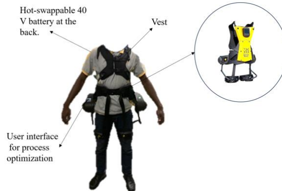
Figure 2: Active (CrayX) back-support exoskeleton.
