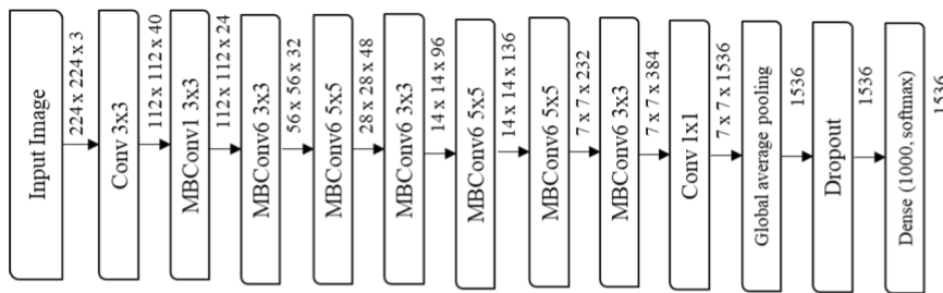
(a) Original EfficientNetB3 architecture diagram
