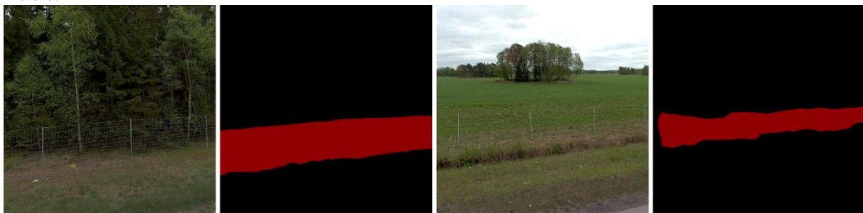
Figure 6. Two samples from the validation pool and their respective predictions. The red color indicates pixels that have been identified as game fence by the FCN.
