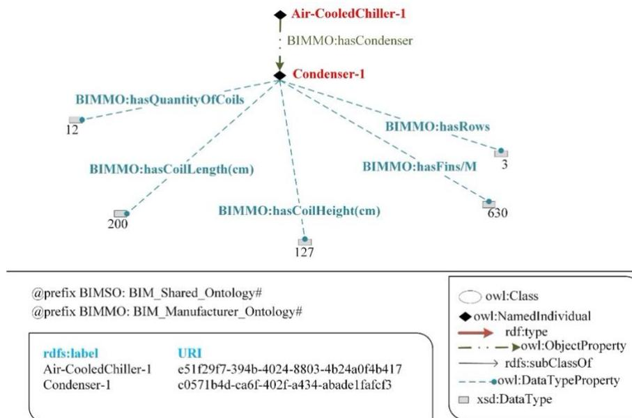
FIG. 13: A chiller's condenser properties
