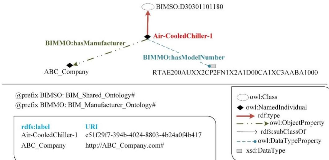
FIG. 5: A chiller's manufacturer and model number
