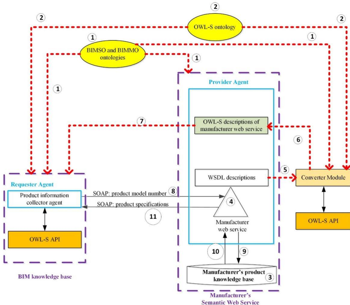
FIG. 2: A schematic view of the Communication between a BIM knowledge base and a manufacturer Semantic Web Service (SWS)
