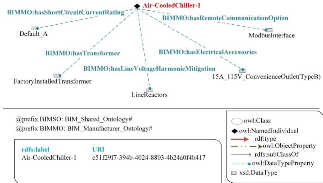
FIG. 10: A chiller's short circuit current rating, transformer, voltage mitigation, electrical accessories, and remote communication
