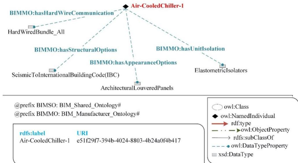
FIG. 11: A chiller hardwire communication, structural option, appearance, and unit isolation
