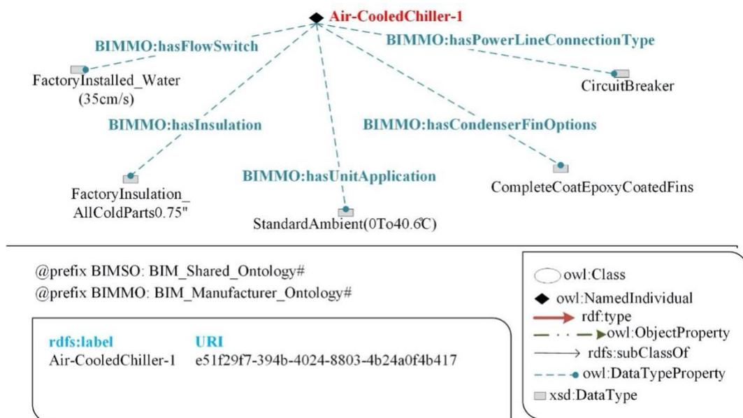
FIG. 9: A chiller's flow switch, insulation, unit application, condenser fin options, and power line connection type
