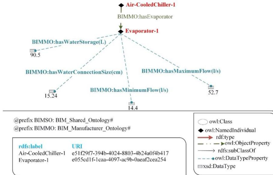
FIG. 12: A chiller's evaporators properties
