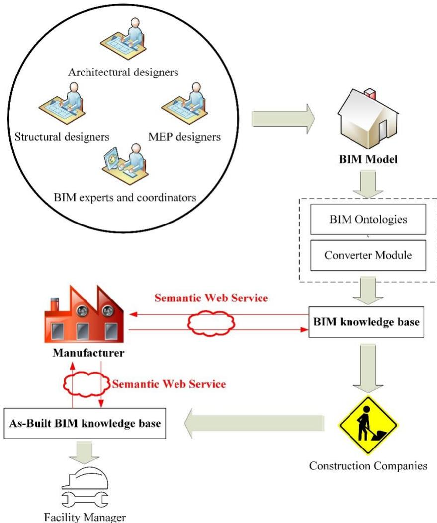
FIG. 1: Using Semantic Web Services (SWS) to integrate manufacturer product data with the BIM data.
