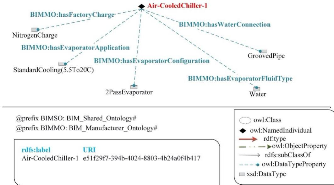
FIG. 8: A chiller's factory charge, evaporator application, evaporator configuration, evaporator fluid type, and water connection
