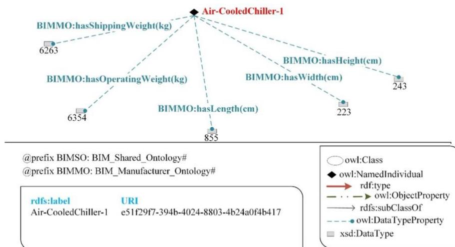
FIG. 15: A chiller's weight and dimensions
