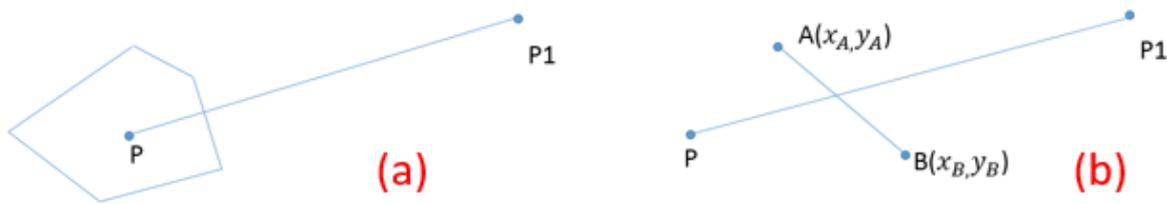
FIG. 5: (a) Deciding whether the user point is inside the given room or not; (b) Deciding whether two segments intersect with each other or not
