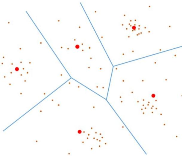
FIG. 3: An illustrative example of K-means clustering
