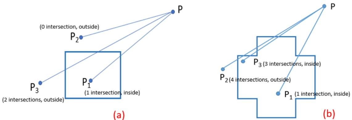
FIG. 6: (a) Example of room identification with a rectangular room; (b) Example of room identification with an irregular room
