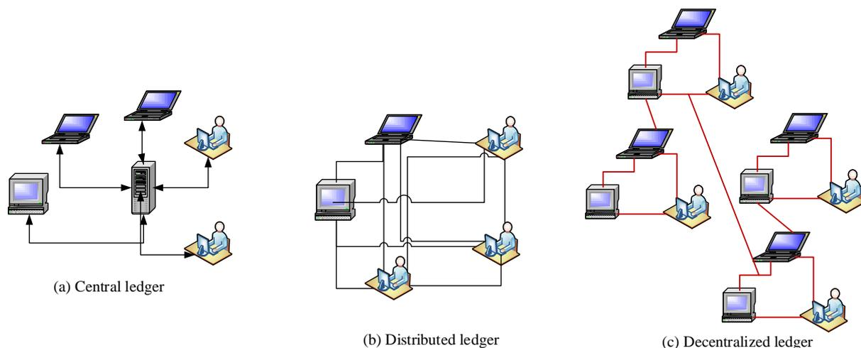
FIG. 4: Different types of network architectures.
