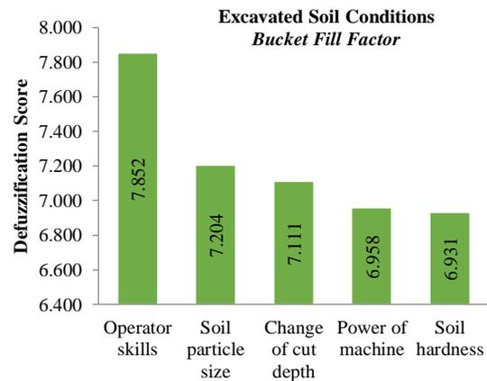
Figure 7: Ranking Scores of Excavated Soil Conditions-Bucket Fill Factor
