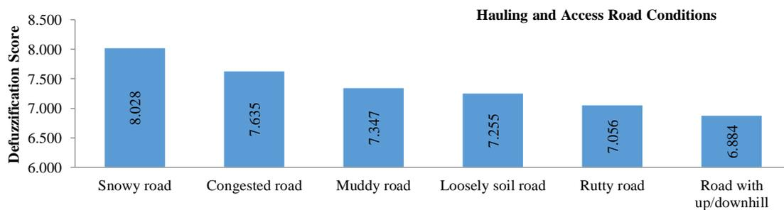
Figure 8: Ranking Scores of Hauling and Access Road Conditions
