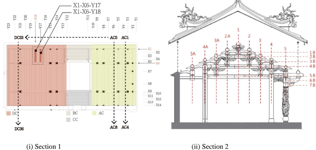
FIG. 2. Sections of the Huchi Tem illustrating the classification and coding system (Ma et al. 2016).
