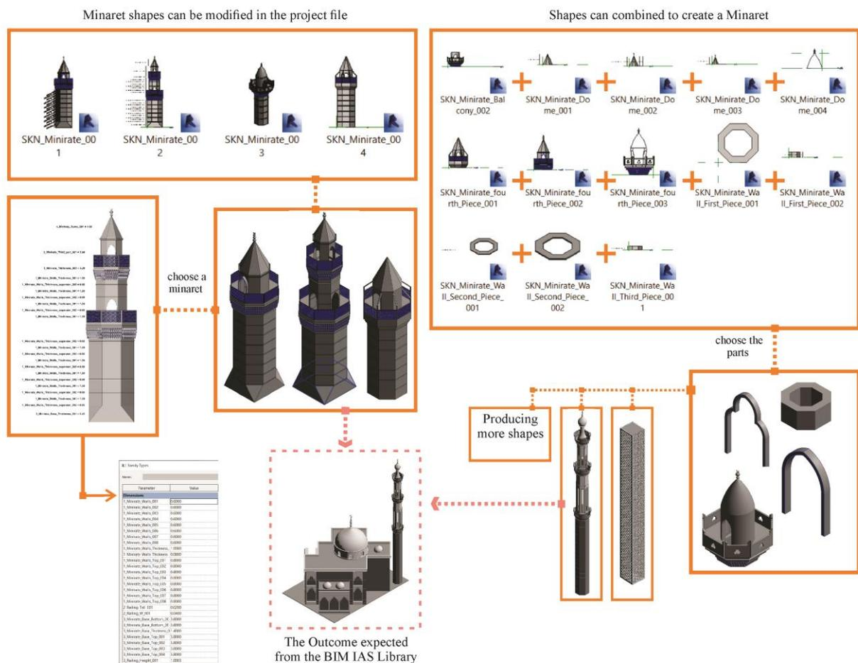
FIG. 6. The complete component and separated parts of HIAC minaret.
