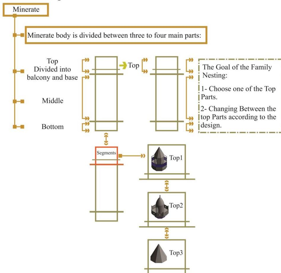
FIG. 8. Hierarchal nested components of the Minaret of HIAC components digital library.
