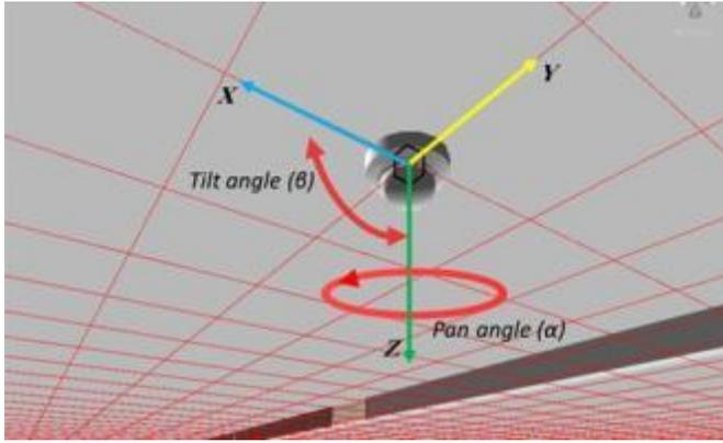
Figure 7: Camera orientation and the 2D grid in BIM
