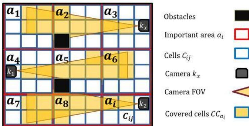
Figure 10: Example of coverage calculation (adapted from Albahri and Hammad, 2015)
