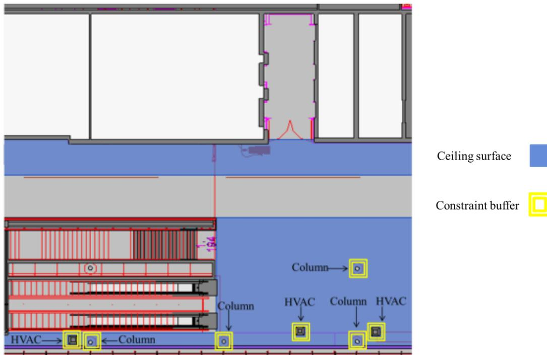
Figure 12: Defining the valid positions for the camera placement using BIM
