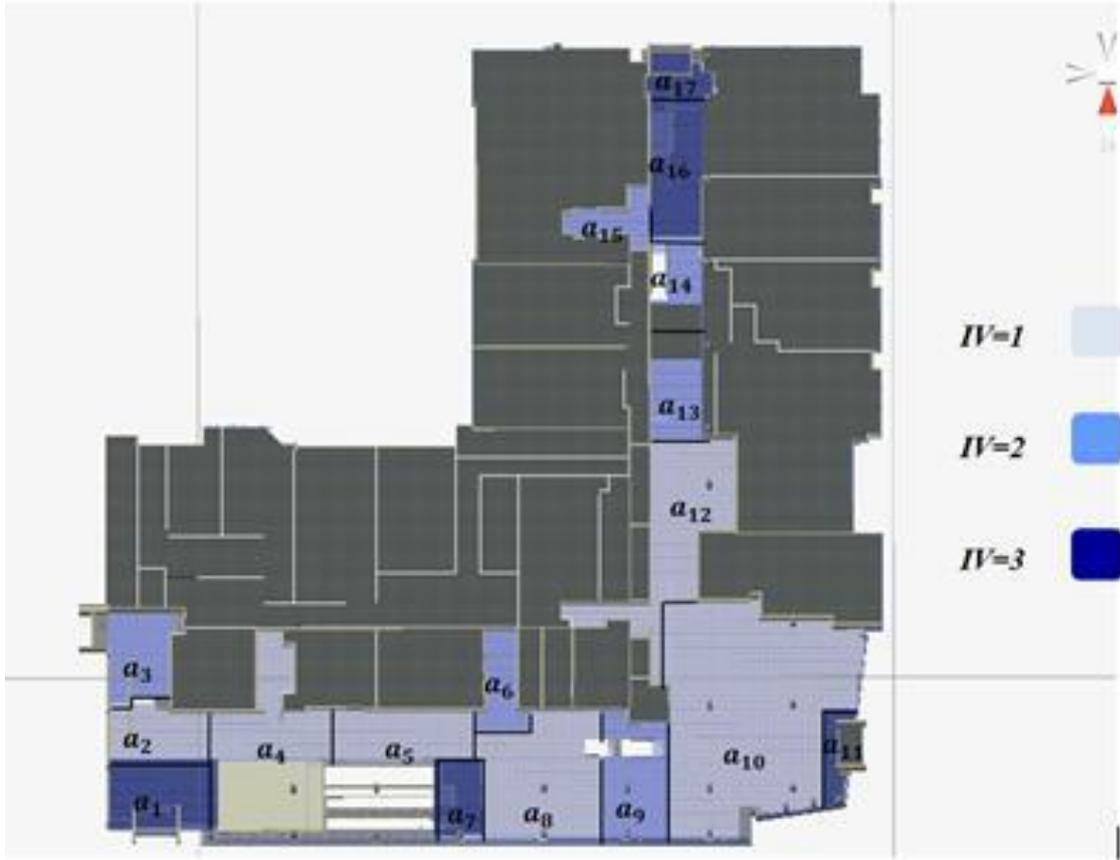
Figure 13: Plan view of the BIM model showing the important areas with their Importance Values (IV)
