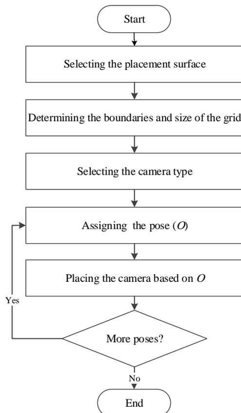
Figure 6: Placing camera using 2D grid
