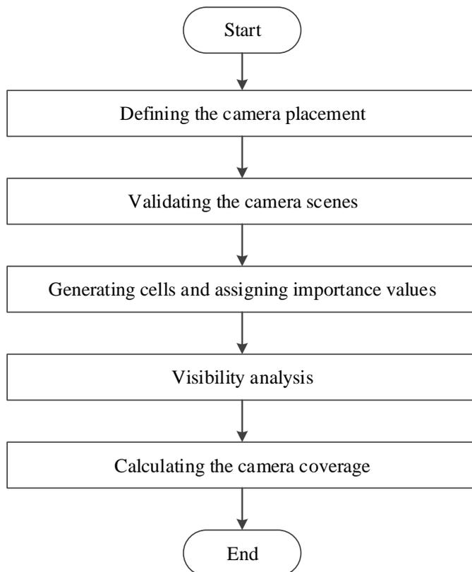
Figure 5: Proposed method for calculating the camera coverage
