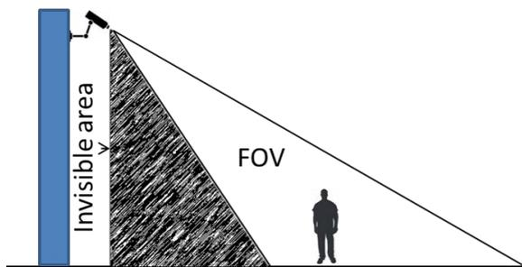
Figure 1: Invisible area under the FOV of the camera (Albahri and Hammad, 2015)
