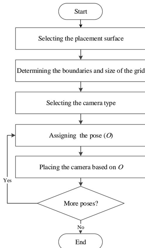
Figure 6: Placing camera using 2D grid
