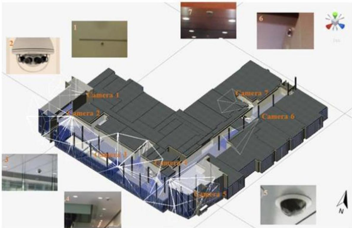
*Figure 11: BIM model aligned with FOVs in the game engine*
