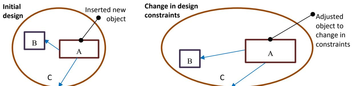
Figure 5: Principles of smart objects and response to update of design.
