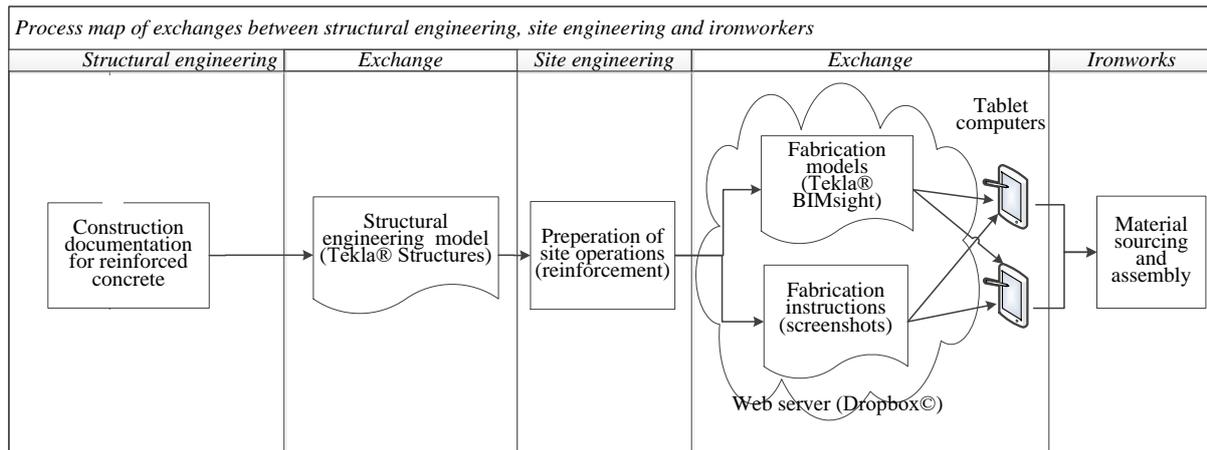
FIG 3. Concrete reinforcement model data exchange in the Oslo Terminal 2 case study
