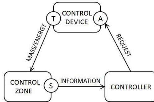
FIG 1: A basic control loop involving a control device, a control zone, and a controller. "T" and "A" denote device's terminal and actuator, whereas S stands for sensor
