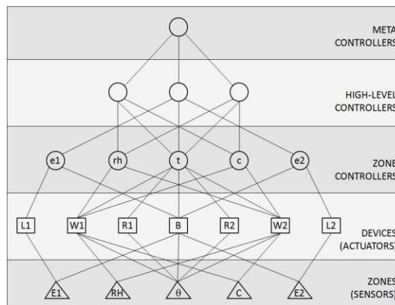
FIG 4: Illustrative distributed multi-layer multi-domain systems control schema for the office space of Fig 3
