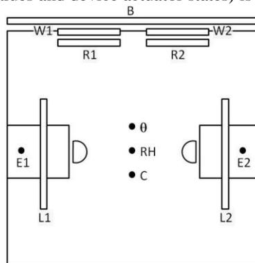
FIG 3: An office space with seven devices (windows W1 and W2, two radiators R1 and R2, two luminaires L1 and L2, and external shade B) and five sensors (illuminance sensors E1 and E2, indoor air temperature, relative humidity, and carbon dioxide sensors  $\theta$ , RH, and C)
