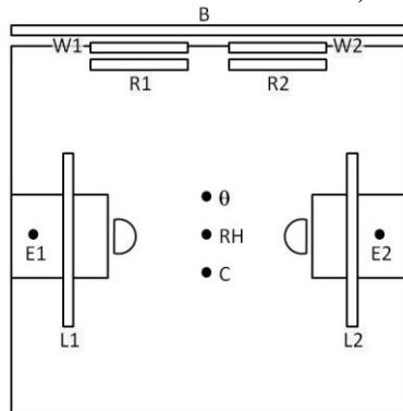
FIG 3: An office space with seven devices (windows W1 and W2, two radiators R1 and R2, two luminaires L1 and L2, and external shade B) and five sensors (illuminance sensors E1 and E2, indoor air temperature, relative humidity, and carbon dioxide sensors  $\theta$ , RH, and C)
