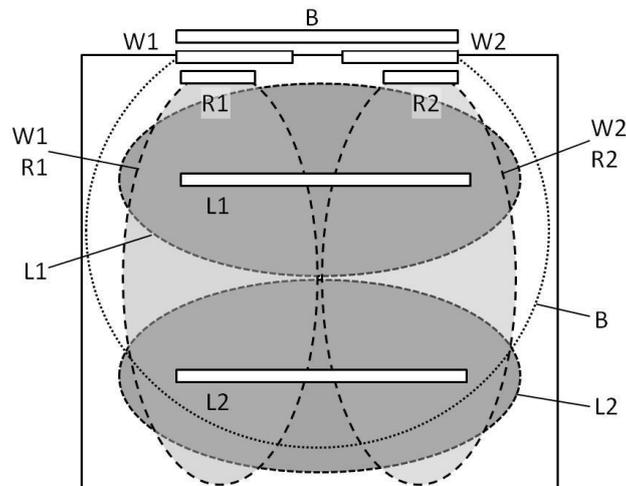
FIG 2: Schematic illustration of a room with multiple devices (B: external shade; W1, W2: windows, R1, R2: radiators; L1, L2: luminaires) together with the schematic depiction of the associated control zones
