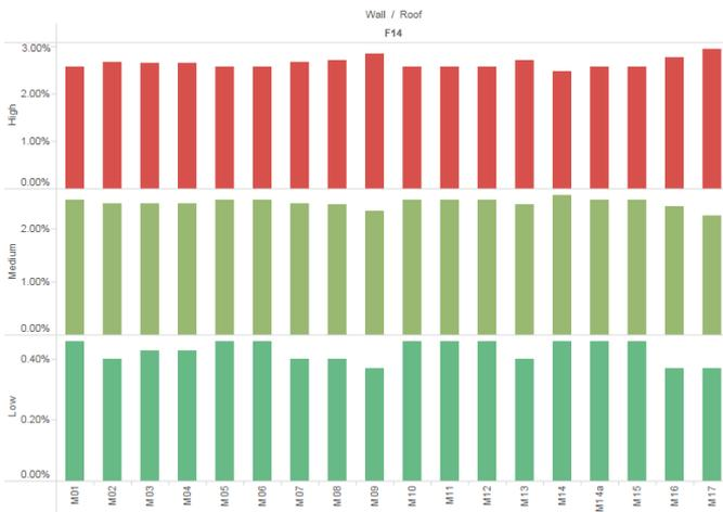
FIG. 19: The possibility of each roof material with the selected wall material (F14) for the three levels of energy consumption.
