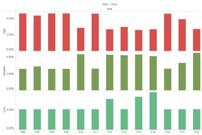
FIG. 18: The possibility of each floor material with the selected wall material (F14) for the three levels of energy consumption.
