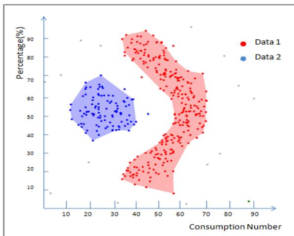
FIG. 4: Density-based spatial clustering of applications with noise (DBSCAN).
