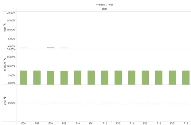
FIG. 21: The possibility of each wall material with the selected window material (Blue 6MM) for the three levels of energy consumption.
