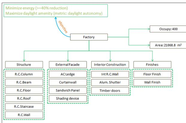
FIG. 11: Baseline building model parameters.
