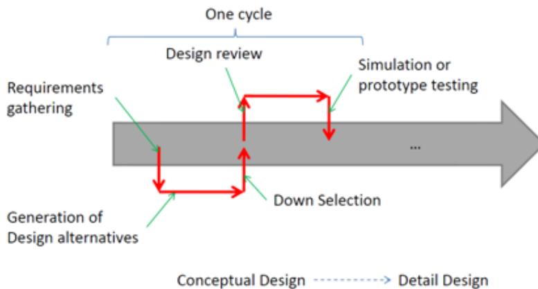
FIG. 2: Overview of the data-driven workflow cycle within the integrated design process.
