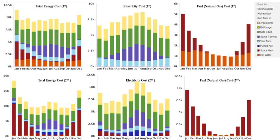
FIG. 9: Monthly cost analysis results for Total Energy, Electricity and Fuel (Natural Gas) for two design options
