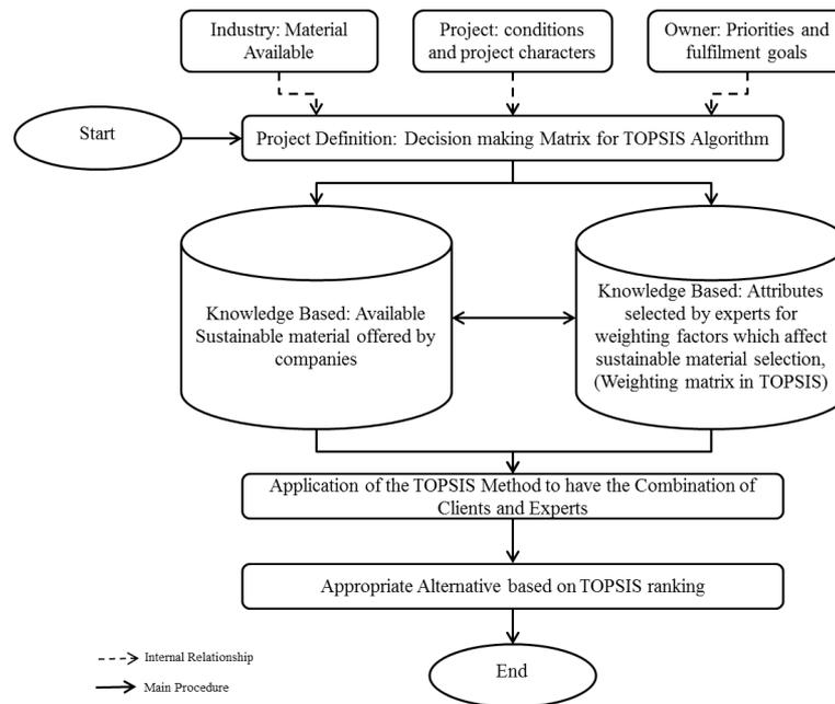
FIG. 3: Decision Support System Schema using TOPSIS algorithm
