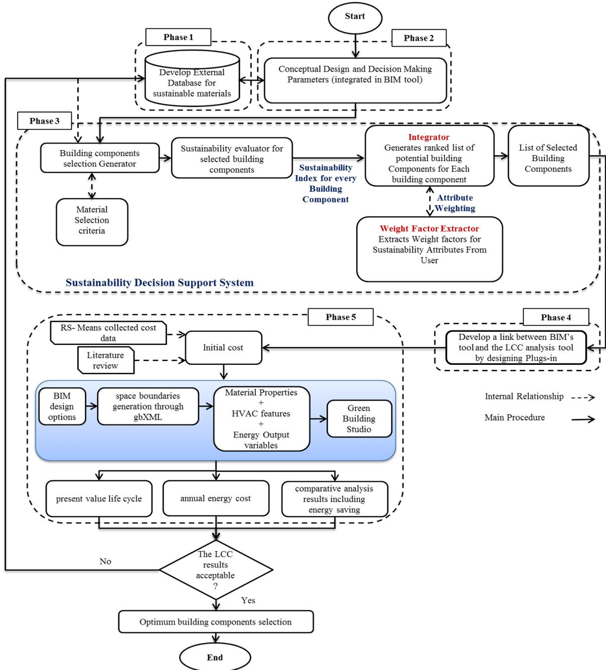
FIG. 1: Flowchart of the integration Process
