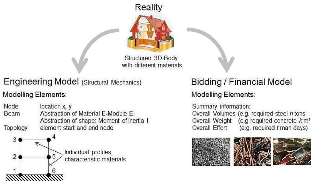
Figure 2: Schema integration (a) by aggregation of structural elements and (b) by decomposition of aggregated values
