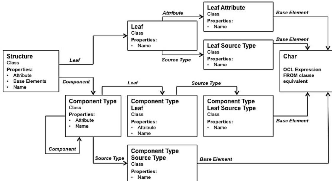
Figure 6: Elements of the model mapping schema (class diagram)
