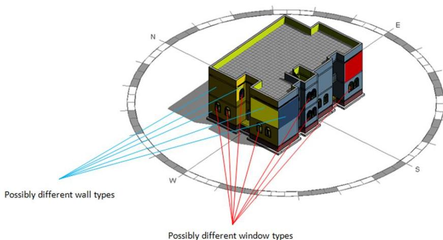
FIG. 5: A perspective of the case study showing the orientation selection and building outer envelope configuration options
