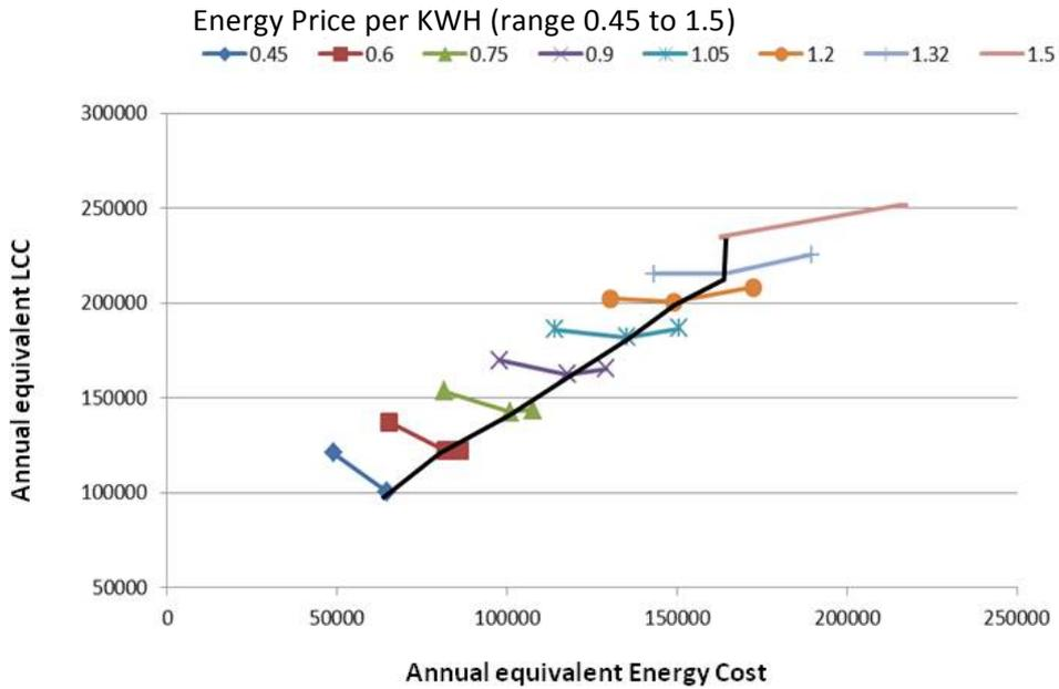
FIG. 7: Optimum LCC Design Contour at various Egyptian Energy prices range from (0.45 to 1.5 LE/KWH)
