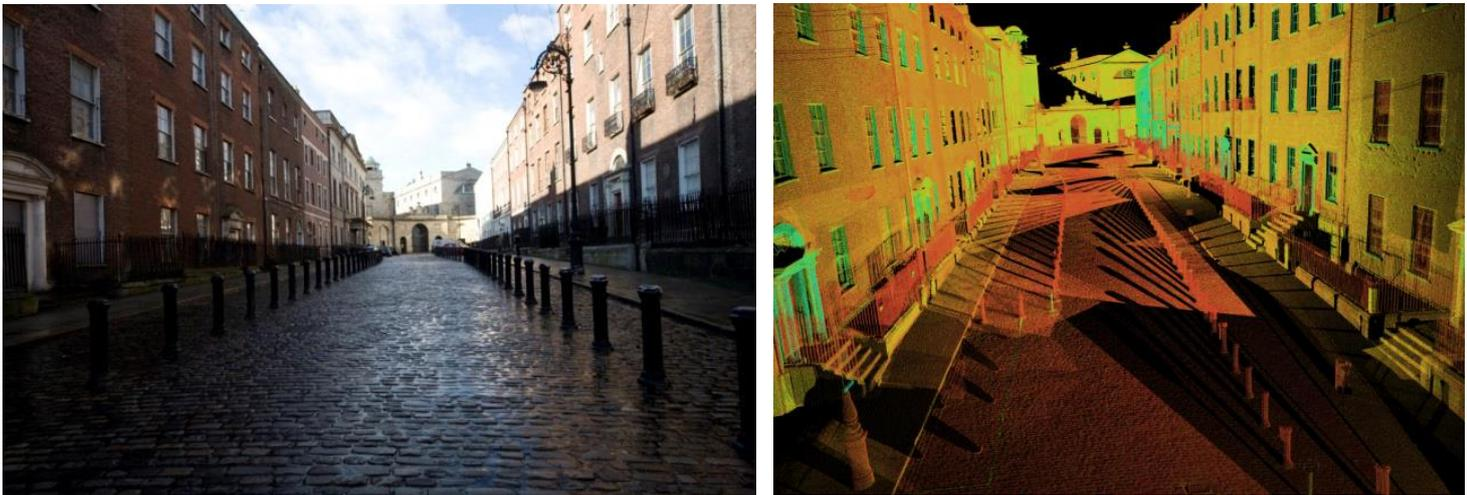
FIG. 20: Henrietta Street, Dublin (left) and point cloud of street coloured by intensity (right).
