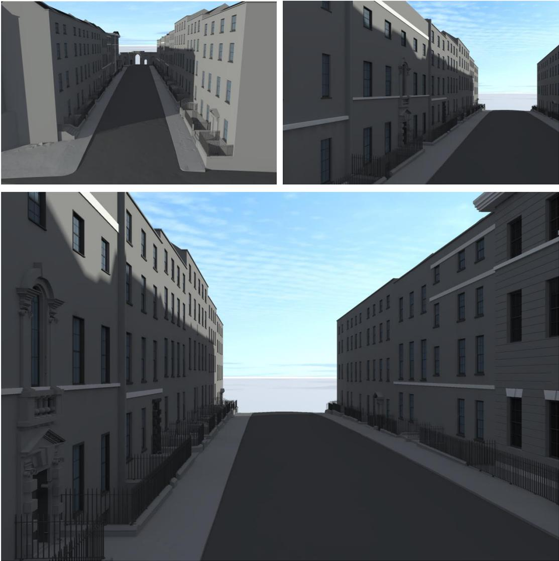
*FIG. 21: BIM model created using HBIM library objects and parametric façade for Henrietta Street, Dublin.*
