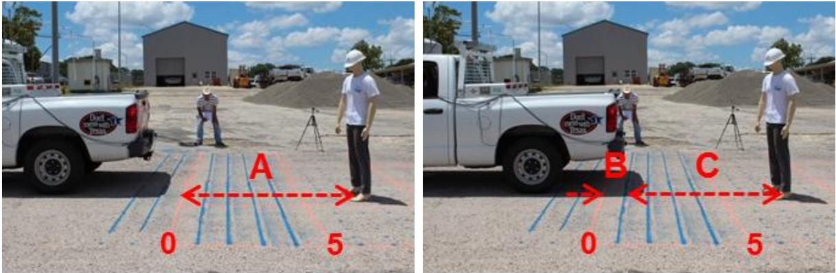
FIG. 7: Basic procedure of the dynamic test. Distance A: Maximum detection range of the sensor in the static condition, Distance B: Range reductions due to the dynamic condition, and Distance C: Dynamic detection range of the sensor in the dynamic condition. The size of each cell is 0.3 by 0.3 meter (1 by 1 foot).
