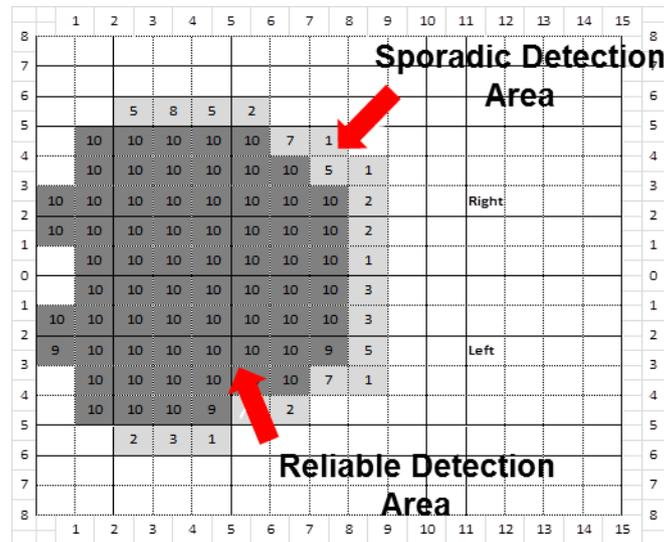
FIG. 5: A sample of the static test data collection. The size of each cell is 0.3 by 0.3 meter (1 by 1 foot).
