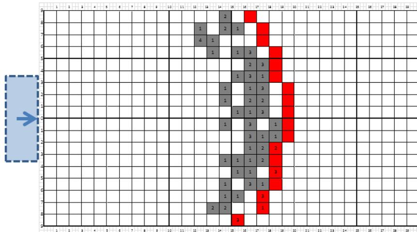
FIG. 12: Dynamic detection zone diagram of system R2 with a pickup truck (Test D3). The size of each cell is 0.3 by 0.3 meter (1 by 1 foot).
