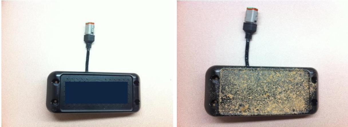
FIG. 10: Dirty sensor test with system R3 - before (left) and after coating (right).
