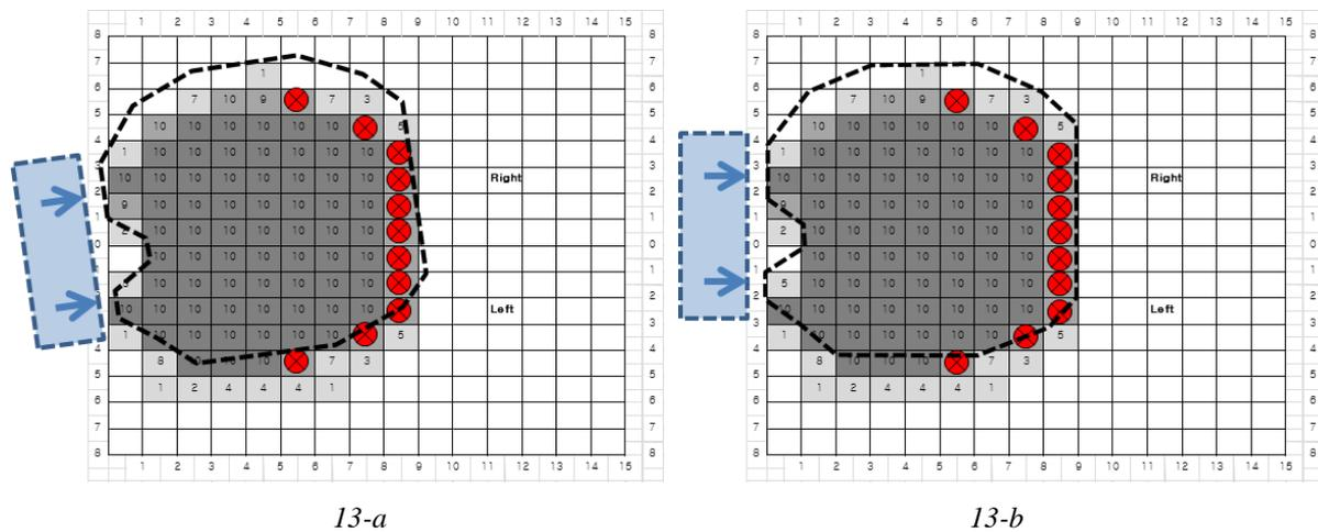
FIG. 13: Example of possible vehicle angle (13- a) and vehicle location (13- b) at zero distance point. The size of each cell is 0.3 by 0.3 meter (1 by 1 foot).
