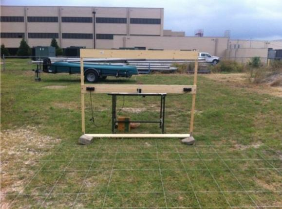
FIG. 3: Frame and measurement grid setup for static tests
