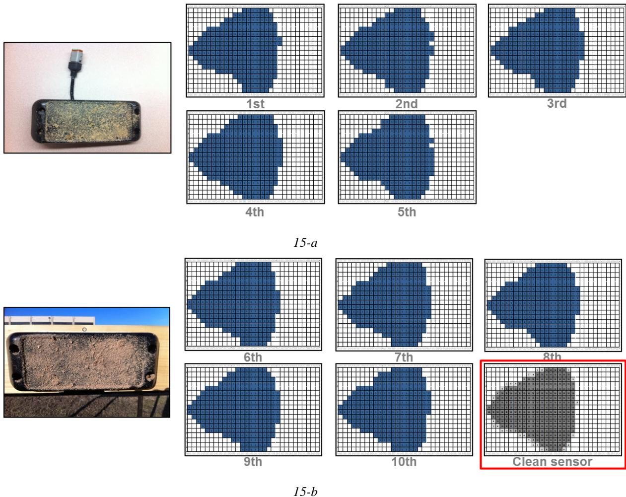
FIG. 15: Dirty sensor test II - Detection zone diagrams of system R3. 1<sup>st</sup> intervention, complete soil coating (14-a) and 2<sup>nd</sup> intervention, 2<sup>nd</sup> layer of soil (14-b). The size of each cell is 0.3 by 0.3 meter (1 by 1 foot).
