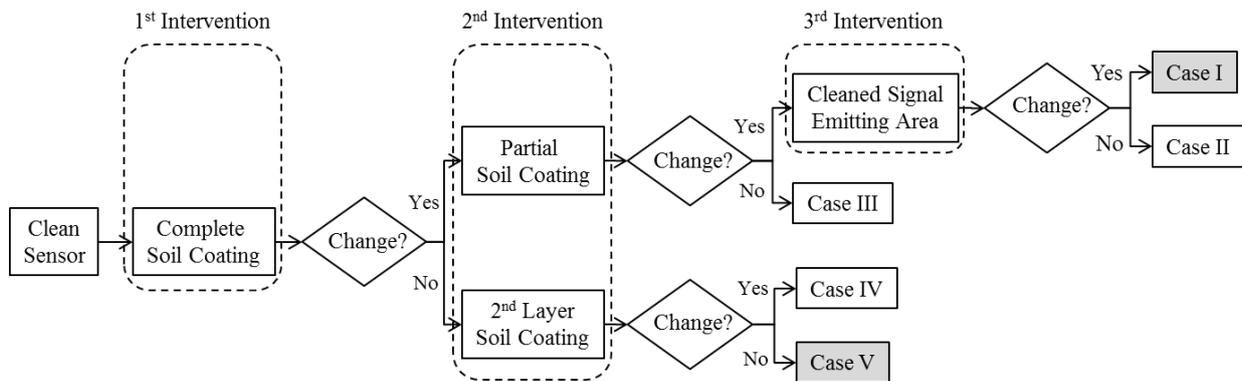
FIG. 9: Process diagram of dirty sensor test
