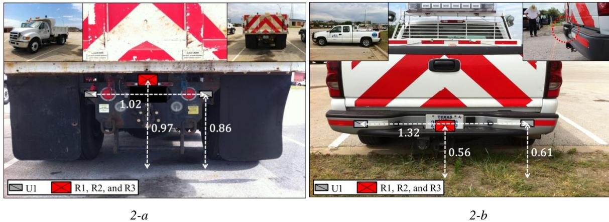
FIG. 2: Sensor installation survey. Installation survey with dump truck (2-a) and Installation survey pickup truck (2-b)
