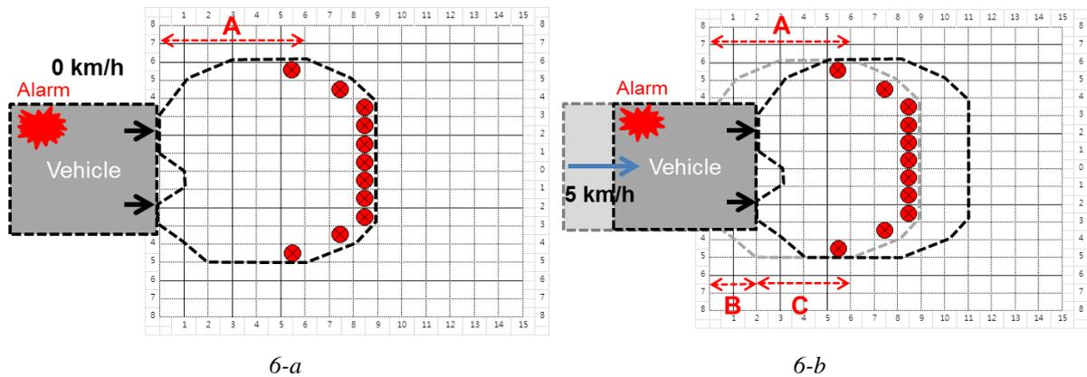
FIG. 6: Detection range model. Static test model (6-a) and dynamic test model (6-b). Distance A: Maximum detection range of the sensor in the static condition, Distance B: Detection range reduction due to the dynamic condition, and Distance C: Dynamic detection range of the sensor in the dynamic condition. The size of each cell is 0.3 by 0.3 meter (1 by 1 foot).
