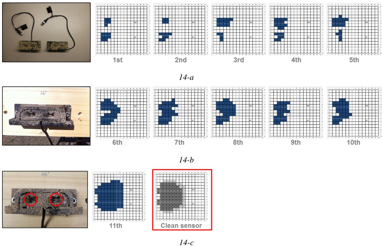
FIG. 14: Dirty sensor test I - Detection zone diagrams of system U1. 1<sup>st</sup> intervention, complete soil coating (13-a), 2<sup>nd</sup> intervention, partial soil coating (13-b), and 3<sup>rd</sup> intervention, signal emitting areas cleaned (13-c). The size of each cell is 0.3 by 0.3 meter (1 by 1 foot).
