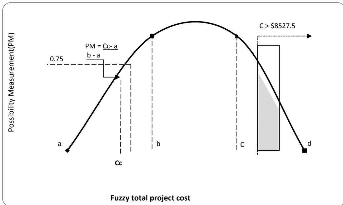
FIG. 6: Fuzzy cost for least cost acceleration plan (scenario 2)
