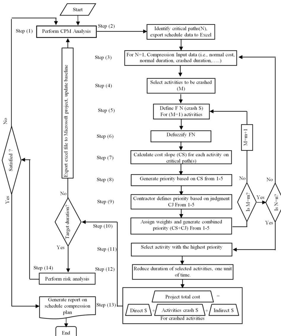
FIG. 1: The flow chart of the proposed method
