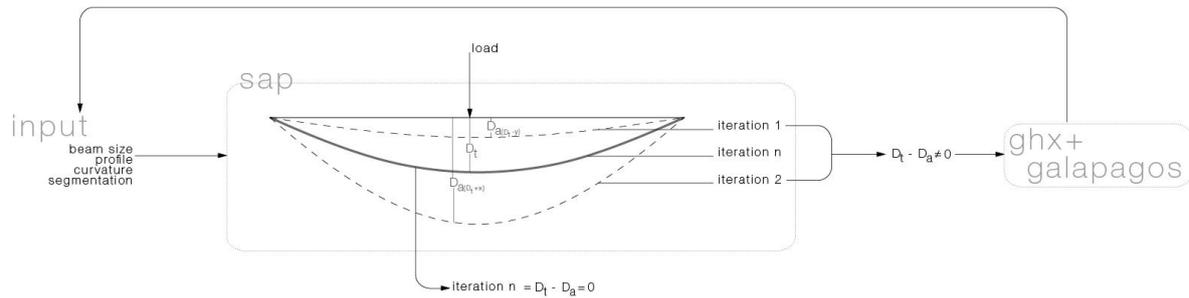
FIG 22: Specified Deflection Diagram
