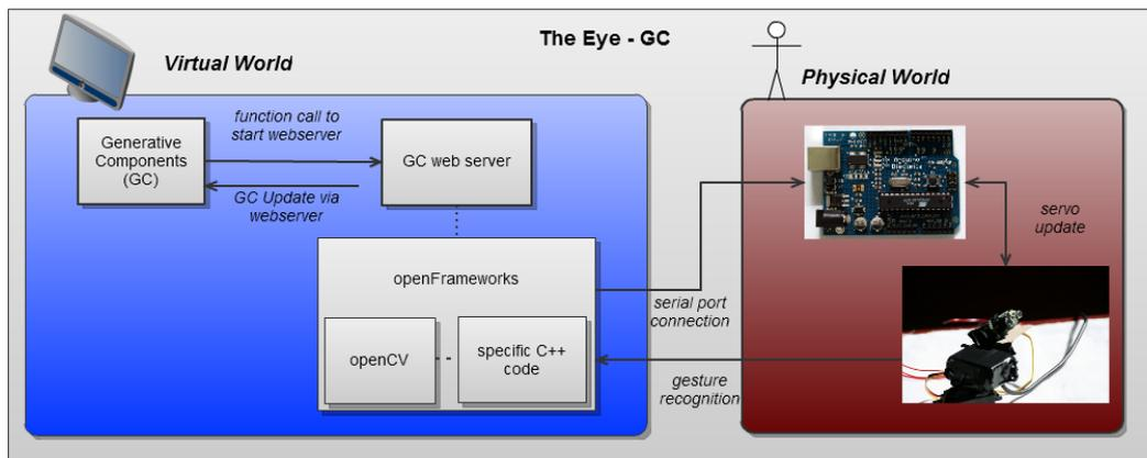
FIG 13: The software architecture of the Eye experiment
