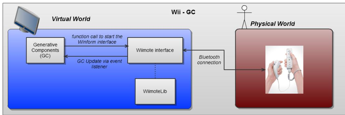
FIG 5: The software architecture of the Wiimote-GC experiment
