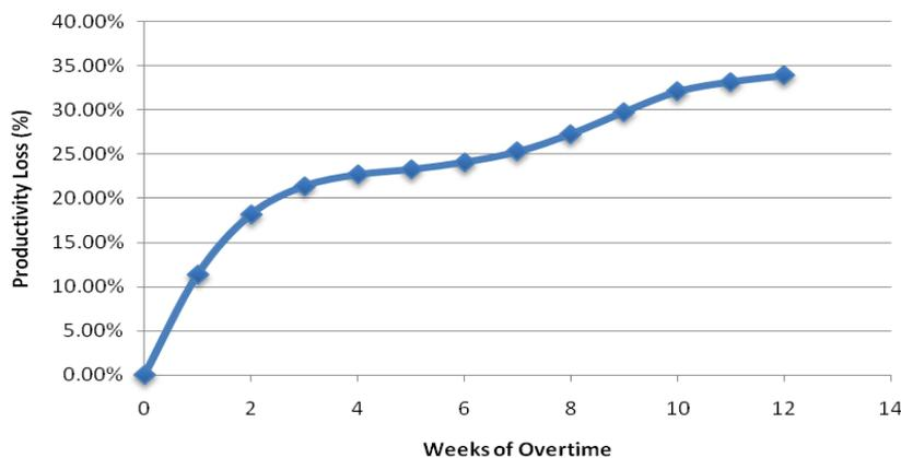
FIG. 4: Productivity Loss due to Overtime based on Hanna and Sullivan (2004)
