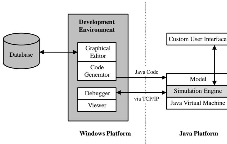
FIG. 6: System Architecture (Modified from Borshchev et al. (2001))
