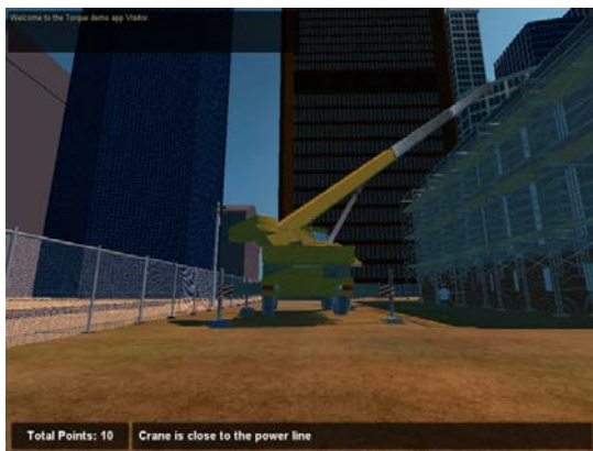
FIG. 1: Point earning with an instructional message when a player correctly identifies that the mobile crane is too close to an overhead power line.
