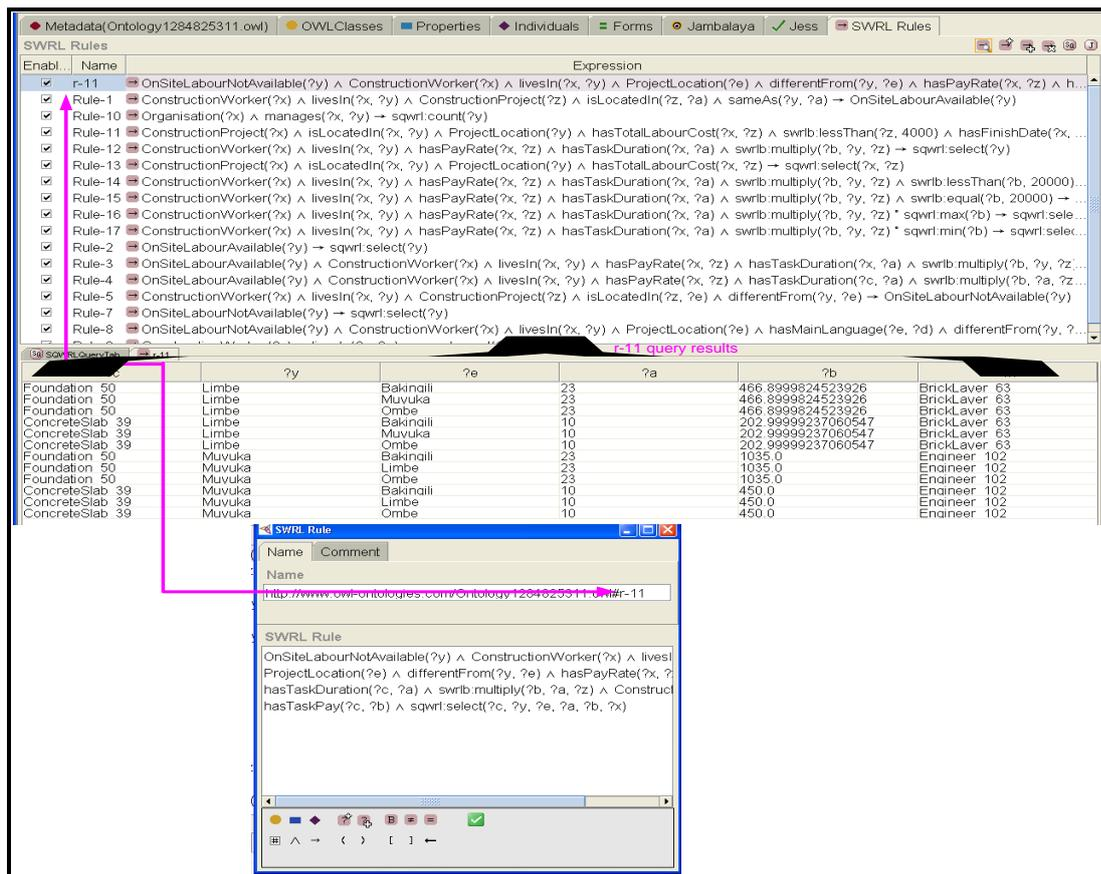
FIG. 4: Labour cost rules in SWRLTab plug-in in protégé-OWL 3.4.4
