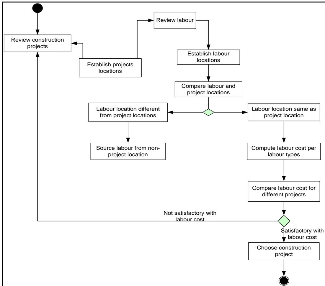
FIG. 2. The process model for the computation of labour cost in building construction in Cameroon
