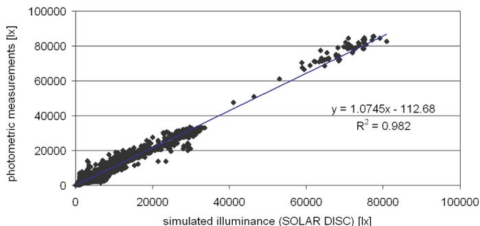
FIG. 3: Comparison of measured external illuminance levels with corresponding camera-based values
