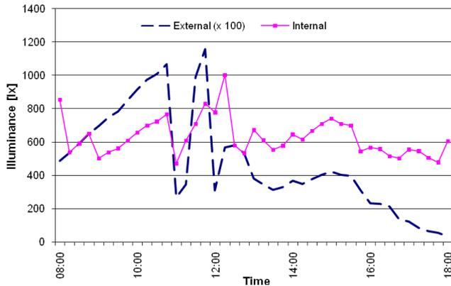
FIG.14: Predicted values of the relevant control parameter (workstation illuminance level) together with the prevailing external global illuminance
