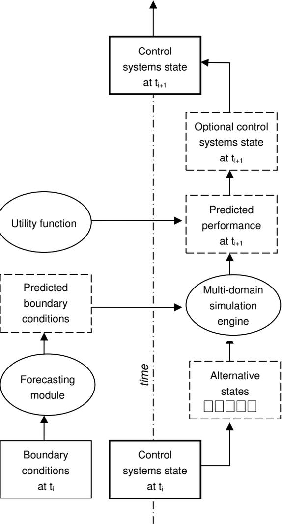
FIG. 1: The schematic illustration of a simulation-assisted building systems control strategy
