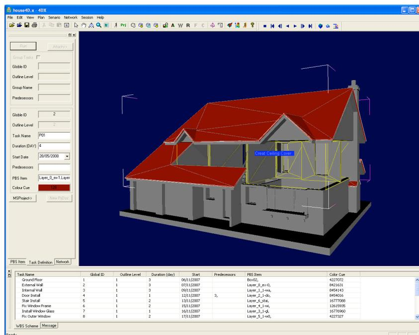
FIG 4: Simulation Item Definition in the 4DX Client Application
