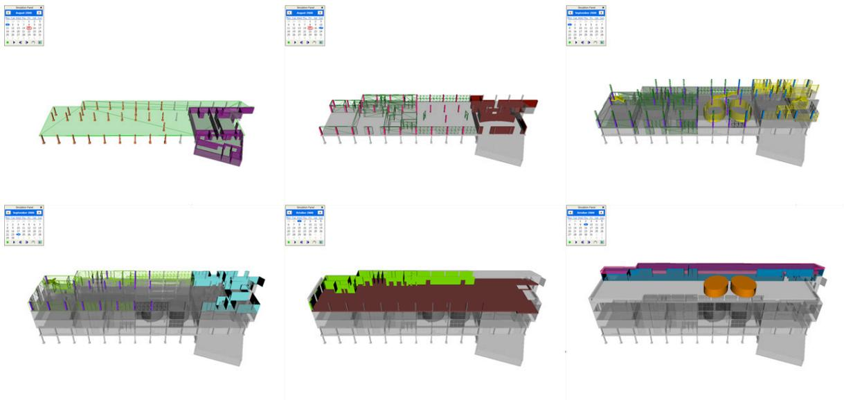
FIG 8: Generated 4D Simulation Sequence in the Testing
