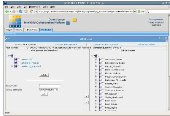
FIG. 8: IntelliGrid testbed portal – GridSphere based portal implementation providing entry point to the available online services (left) and the portlet for managing virtual organisation security settings (right).
