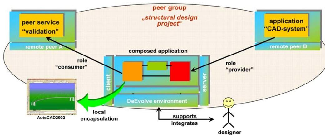
FIG. 2: The DEEVOLVE architecture.
