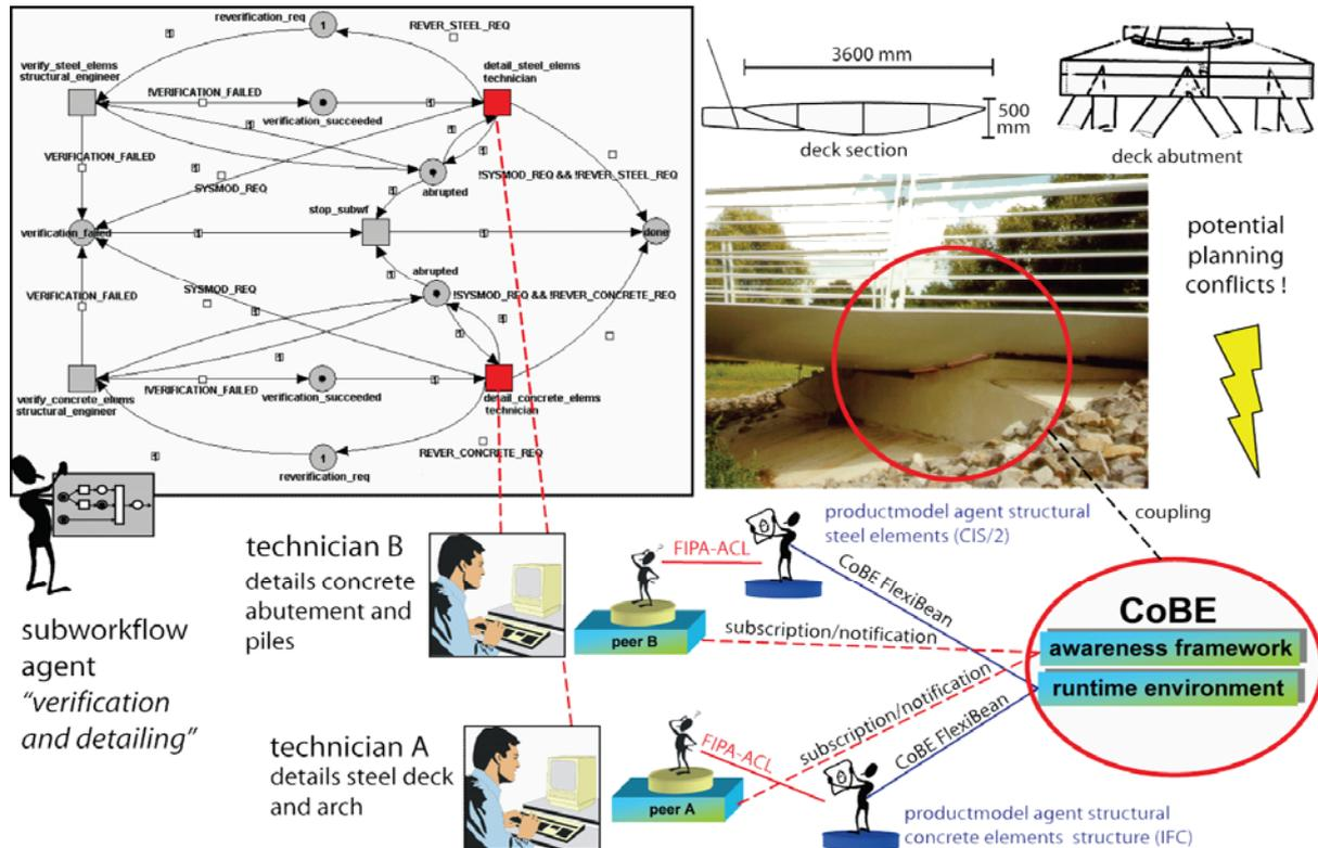
FIG. 8: Subworkflow agent „verification and detailing“ with example detailing scenario.
