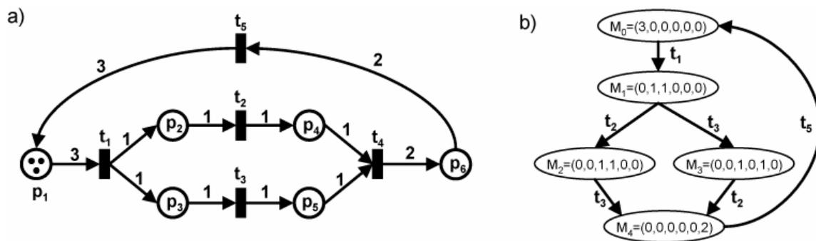
FIG. 4: Simple place/transition (P/T) Petri net with place invariant (a) and related reachability graph (b).
