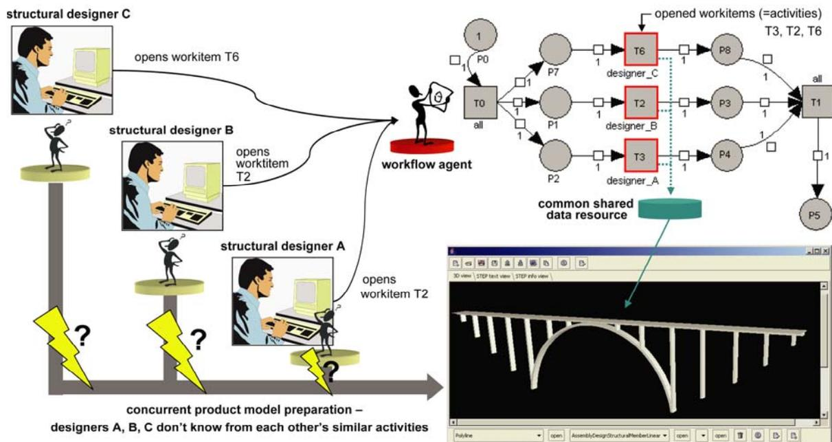
FIG. 5: Conflicting use case: designers A, B and C have to operate on the same bridge model objects concurrently.
