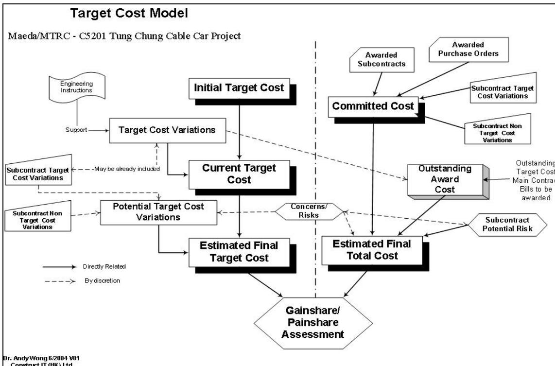
FIG. 4: The target cost model with the elements for the projection to forward looking for decision making during the construction stage.
