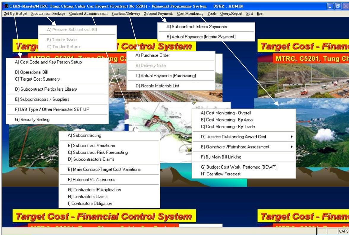
FIG. 3: CIMS-Target Costing main screen with the main functions highlighted.
