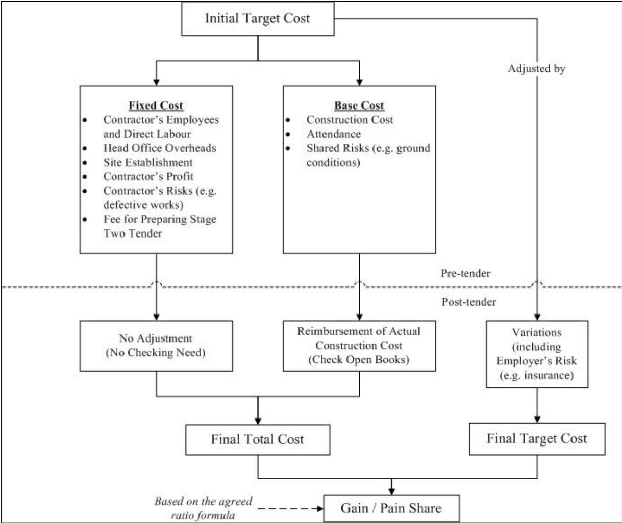
FIG. 1: Gain/Pain Share Mechanism under Target Cost Contracting Arrangement
