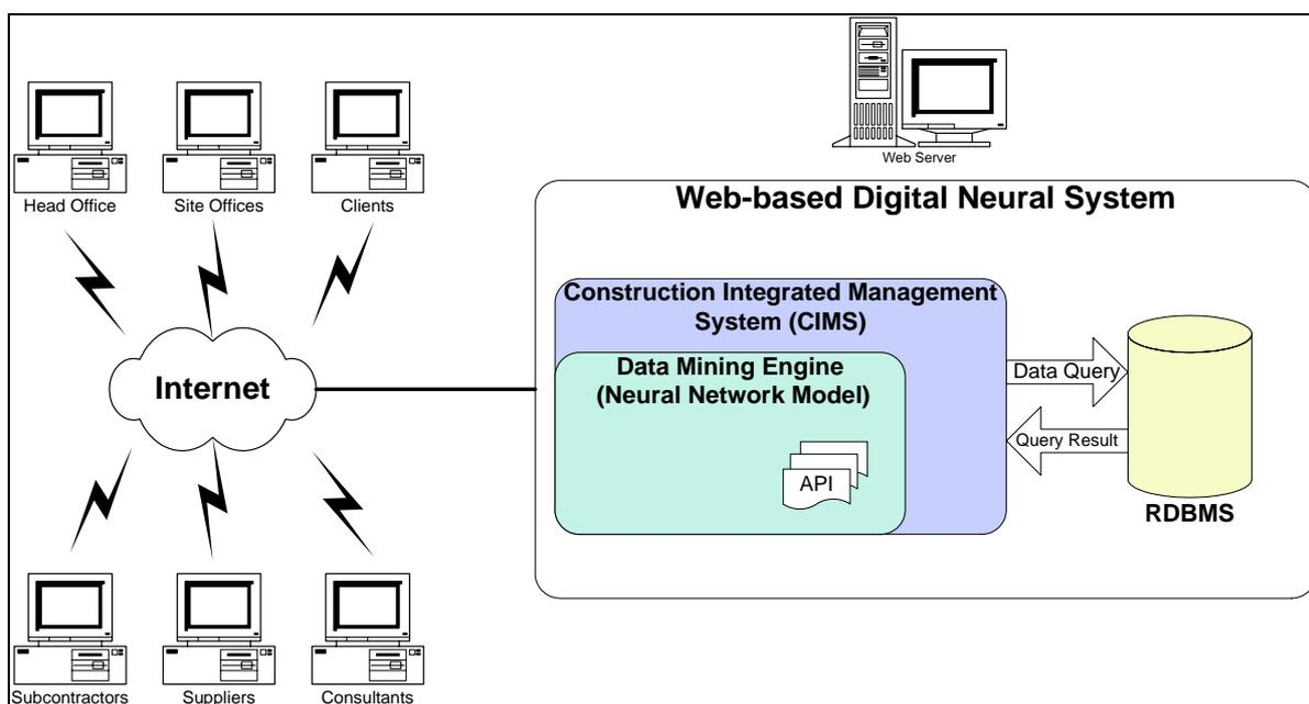
FIG. 8: A prototype of web-based digital neural system for construction project management.
