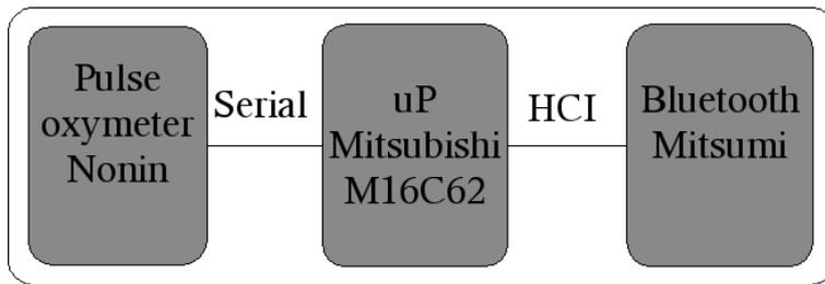
FIG. 6: The EIS test platform architecture. A sensor, in this case a pulse oxymeter, is serially connected to a microprocessor, Mitsubishi M16, running a real time operating system (RTOS) with appropriate parts of the "TCP/IP" suite of protocols and a host controller interface, HCI driver communicating with a Mitsumi Bluetooth 1.1 device.
