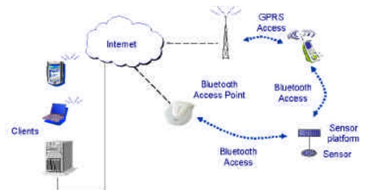
FIG. 4: An EIS device with Bluetooth communication connecting to the Internet via a standard mobile phone or possibly a Bluetooth LAN access point.
