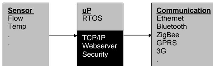
FIG. 3: General architecture of an EIS sensor. A sensor is connected to a microprocessor running a real time operating system (RTOS) with appropriate parts of the "TCP/IP" suite of protocols and drivers for the chosen hardware communication link.
