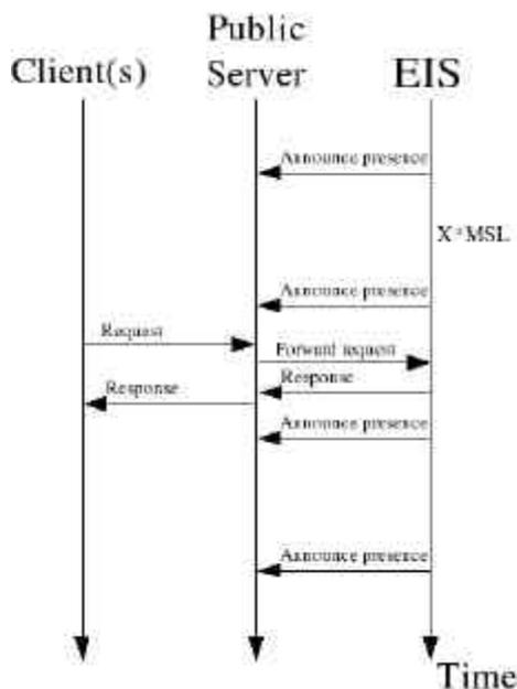
FIG. 5: Connection scheme for announcement and request response of an EIS device. Announcement of presence is made according to the number of Maximum Segment Lifetimes, MSL used by the telecom provider.
