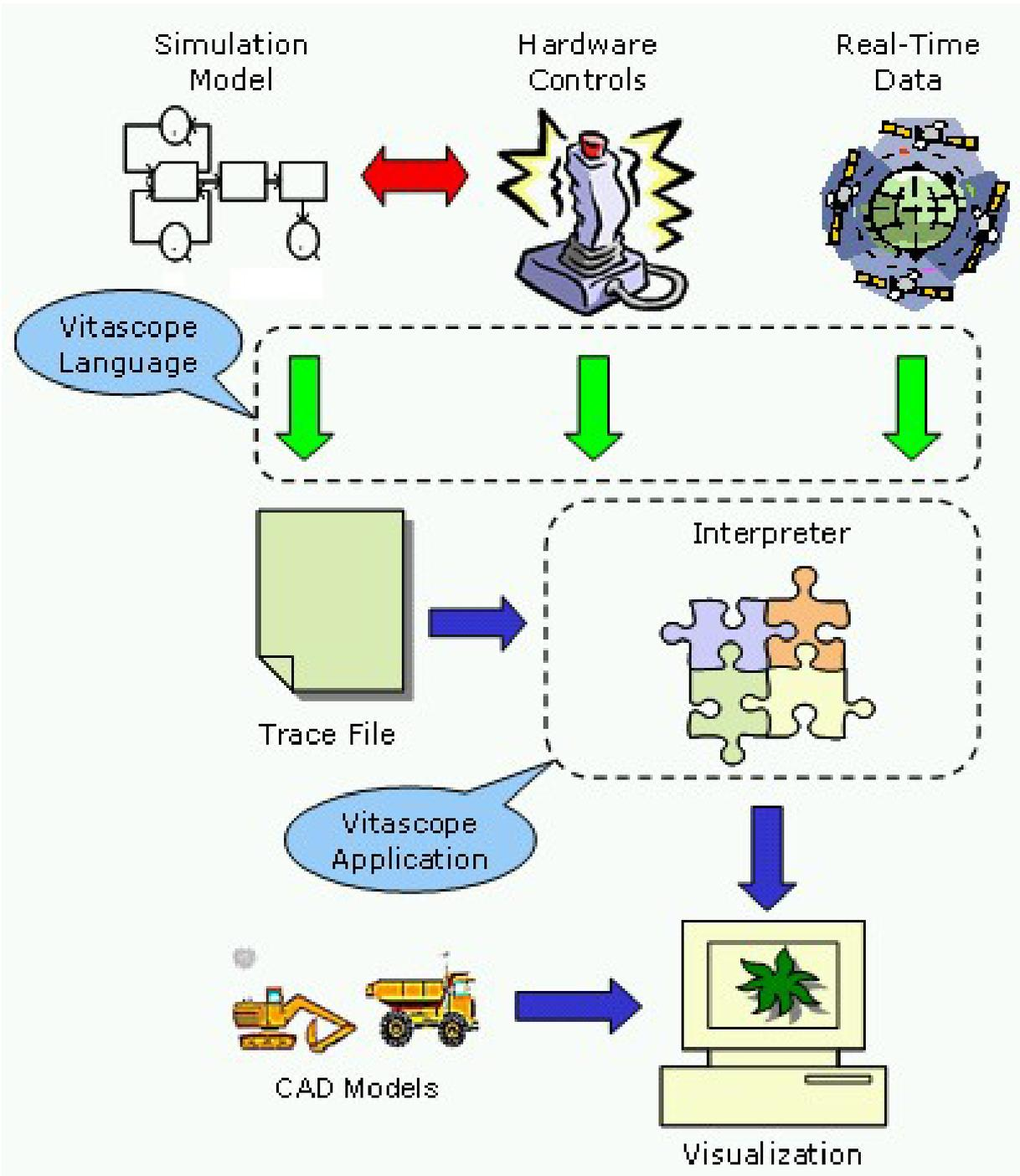
FIG. 1: Relationship between VITASCOPE elements and external authoring processes.
