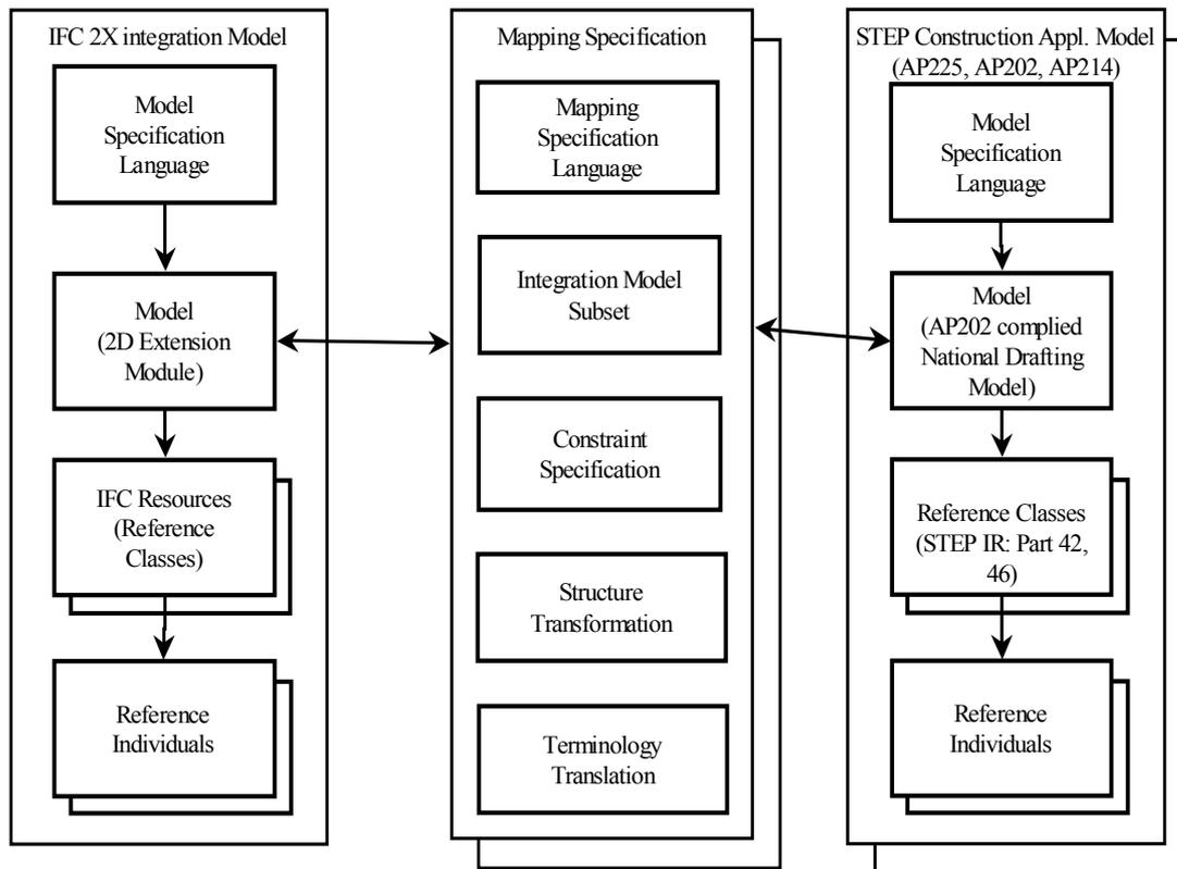
FIG 5: Integration Approach using Mapping methodology [modified from the figure in ISO/TS 18876]
