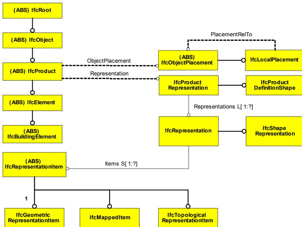
FIG 1: Representation structure in IFC2x
