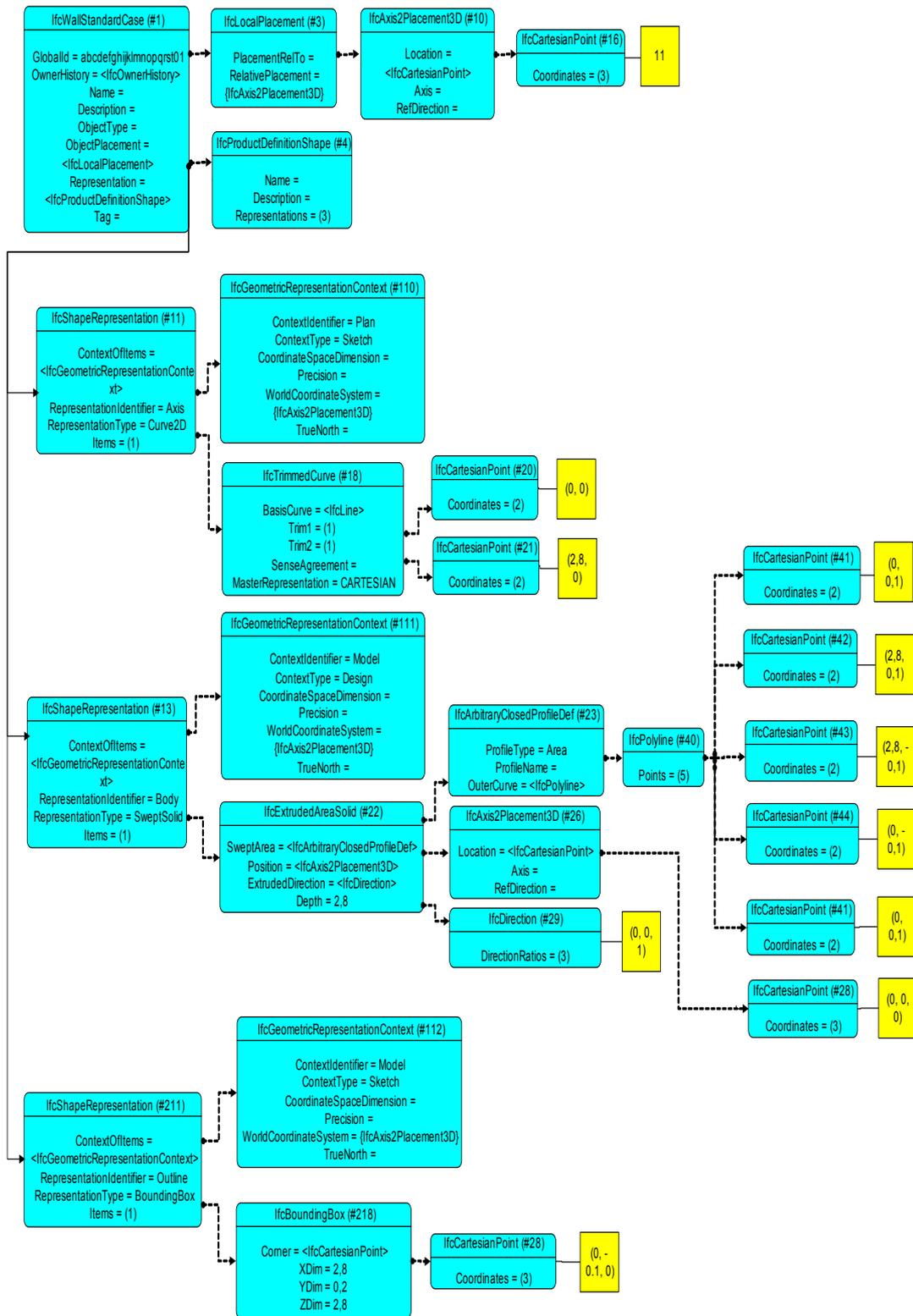
FIG 3: Instance diagram of a multiple representation of a wall
