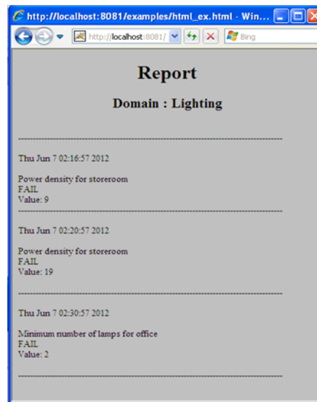
FIG 16: Lighting power density requirement from the EMSD building code (left), and HTML report generated by the Building Code Checking module (right)
