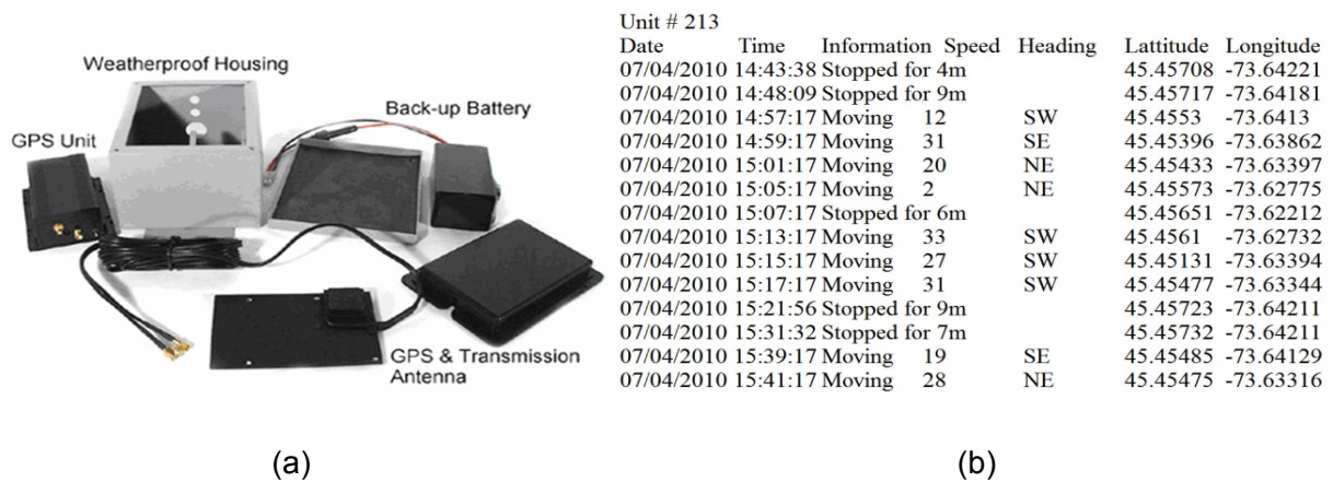
FIG. 2: (a) Main components of the used GPS device (b) GPS raw captured data
