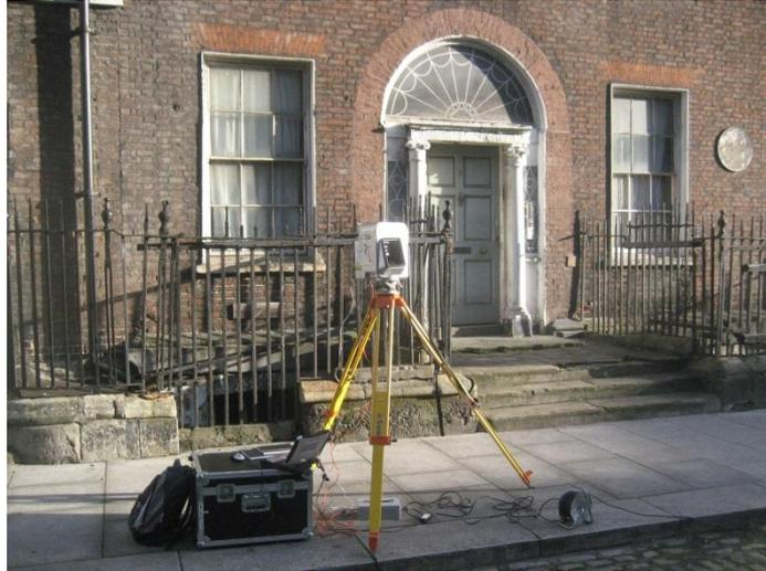
FIG. 19: Trimble GS200 laser scan used to record data for generating as-built BIM model of street.
