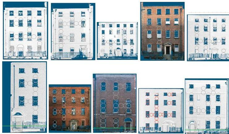
FIG. 3: Testing classical proportions using orthographic images from surveyed classical buildings.
