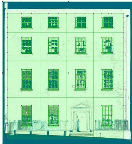
FIG. 17: Orthographic image overlaid with parametric façade template for graphical editing of façade elements.
