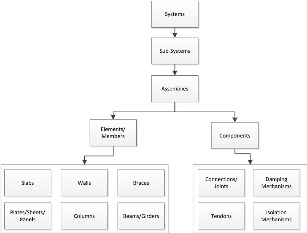
FIG. 3: Assembly to Element Hierarchy Breakdown
