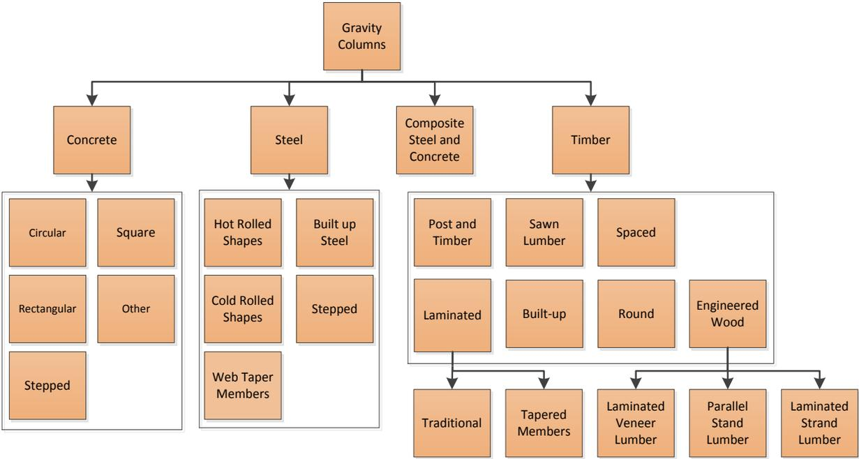
FIG. 4: Material Classes Mapped to a Column Element
