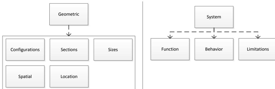
FIG. 10: Constraint Classes: Geometric and System Tree Hierarchies
