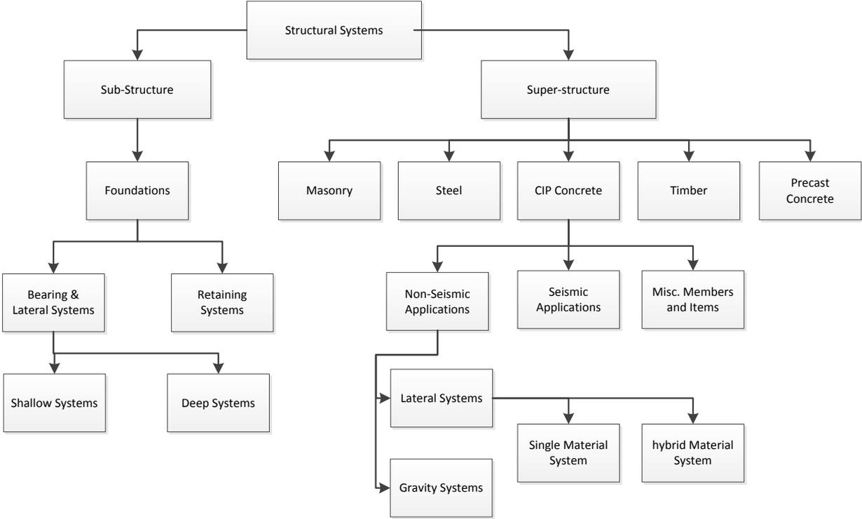
FIG. 2: Structural System Aggregation Template
