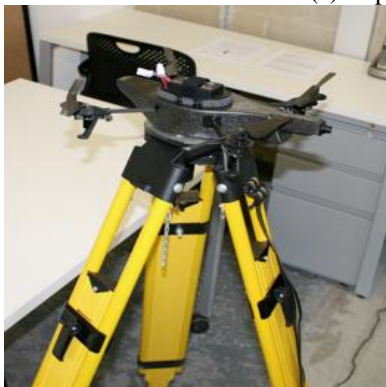
(b) Drone mounted on top of a tripod
