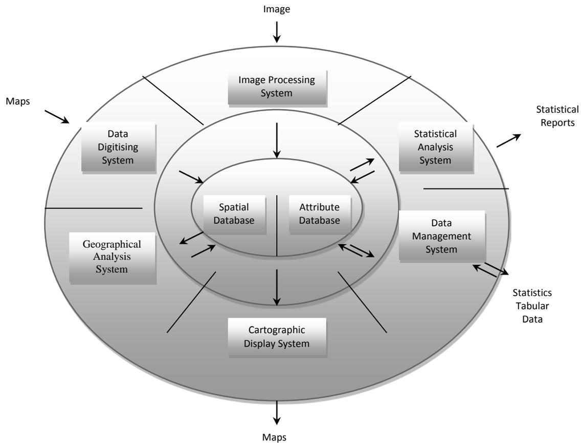
FIG 2: Software Components of a GIS
