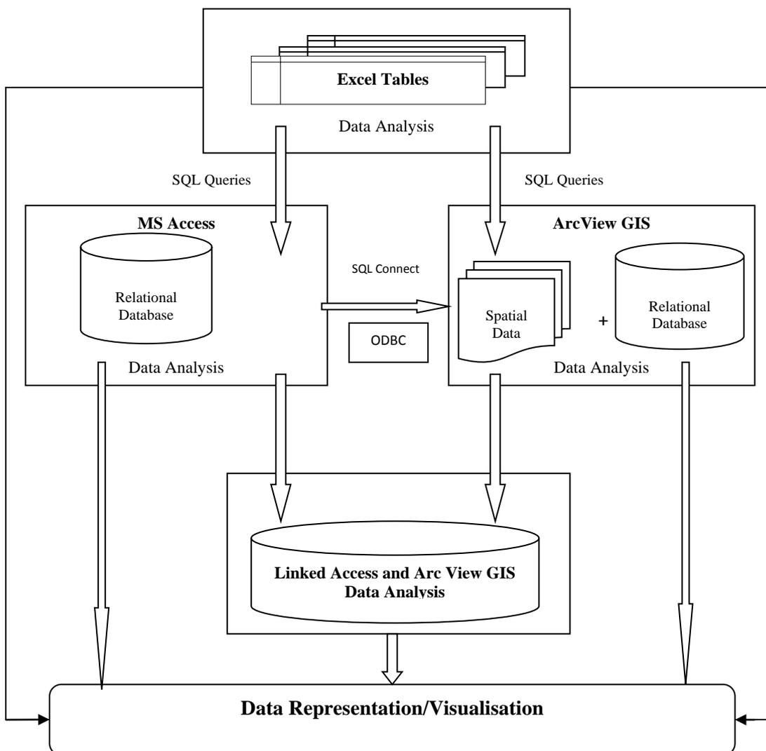
FIG 5: GISAP Analytical System Architecture
