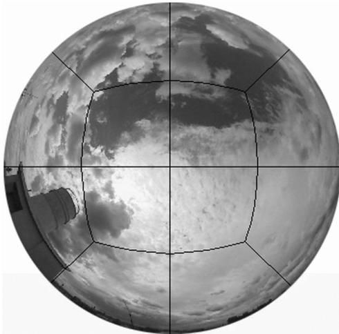
FIG. 2: Fisheye digital image of sky dome (together with the projection of twelve sky sectors as "seen" by illuminance sensors)
