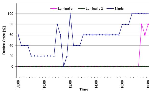
FIG.13: Recommendations (desirable states of lighting and shading devices) of the simulation-assisted lighting and shading control system for a reference day
