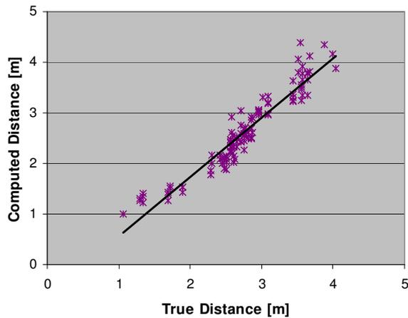
FIG. 8: Actual versus computed tag-camera distances
