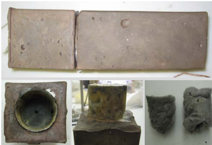
(b) Minor cracks in PTS B1 after test
