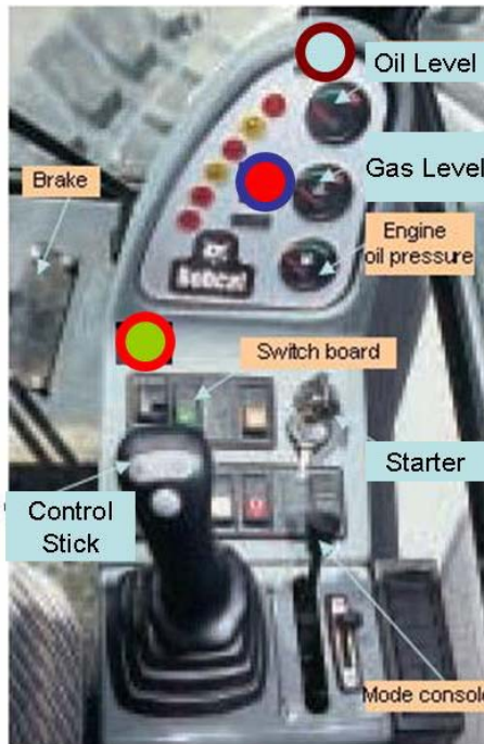
FIG. 3: Hypothetical illustration of augmented instrument panel with corresponding virtual tags positioned via fiducial recognition tracking (Wang et al. 2004).
