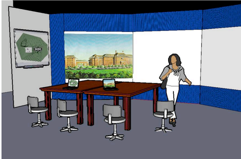
FIG. 12: Layout III: An interactive whiteboard and an additional large screen are used. The interactive whiteboard is used for sketching, with the added screen run from the PC for navigating the 3D model.
