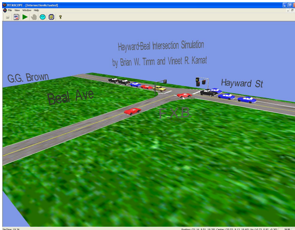
FIG. 9: Traffic Lights Change when Queue Reaches MaxQueueLength
