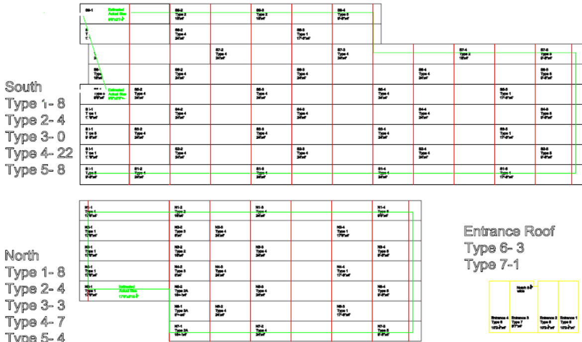
FIG. 12: Layout Drawing for SIPs Panels used in Laser Cutter for Physical Prototype
